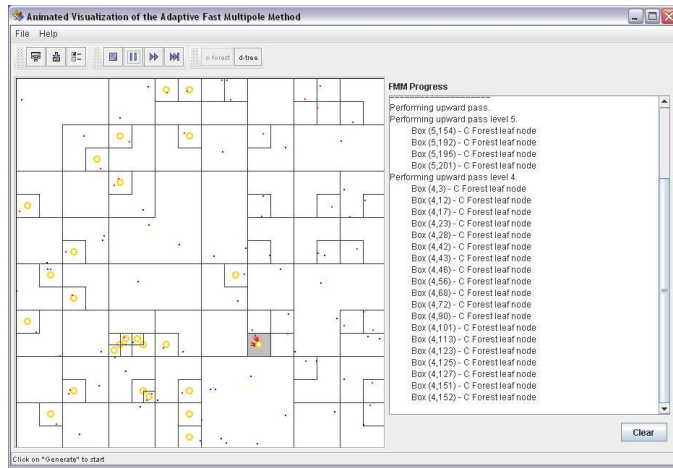
Figure 6.9: Adaptive FMM Algorithm: Upward Pass
