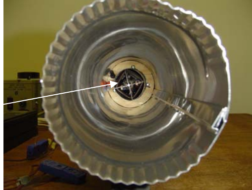
Figure 3.2 Heater mounted within vent pipe
