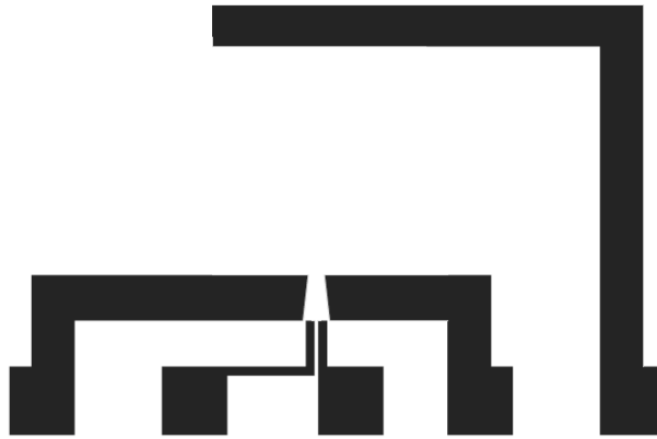
Figure 4.12 Gold lead mask for 5 mm heater
