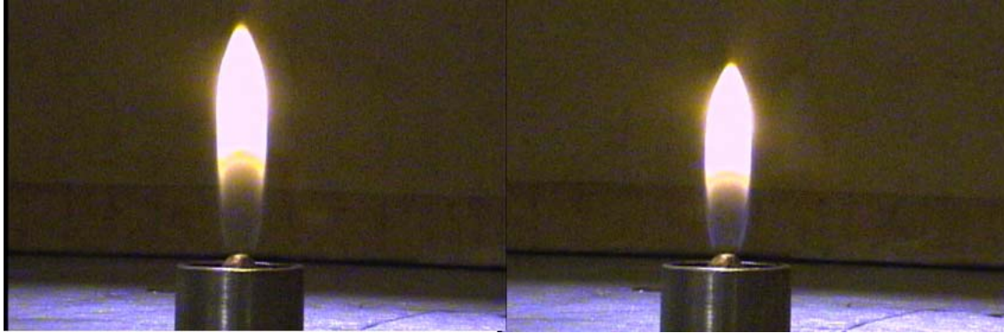
Figure 4.2 Normal Temperature (Left) and Preheated, T = 673 K, (Right) Combustion Air Flame
