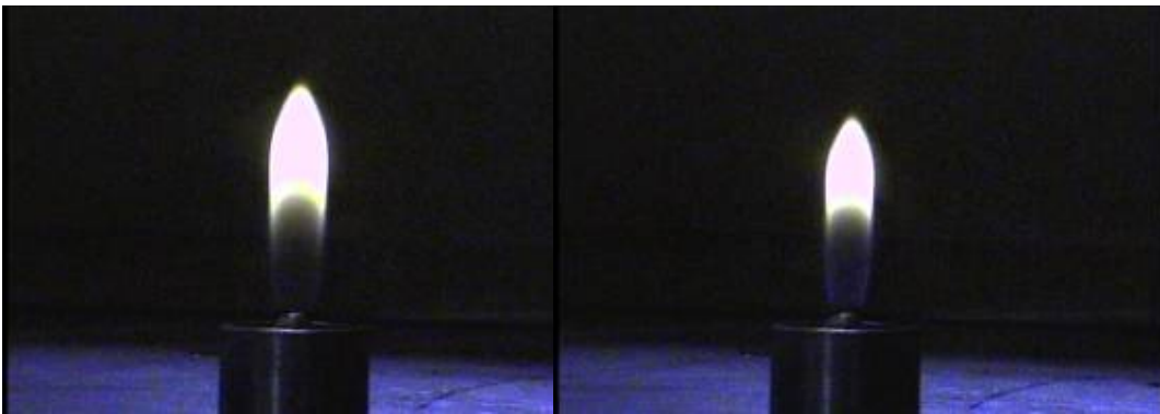
Figure 4.1 Comparison of Laminar Coflow Diffusion Flame Length in Normal-Gravity with Normal (Left) and Preheated Combustion Air (Right) Using CH Filter
