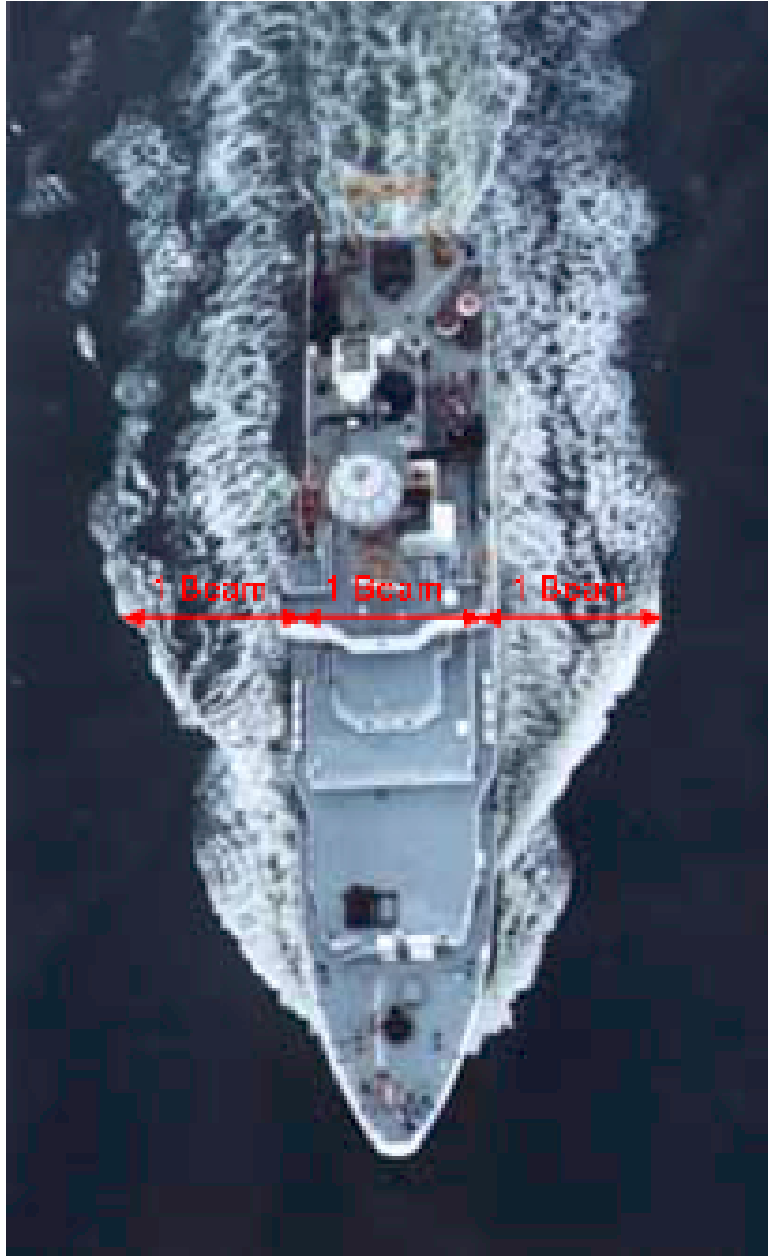
Figure 5.11: A typical wave pattern around a real ship.
