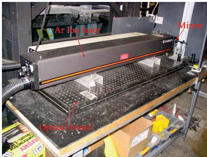
Figure 3.37: A picture of the light source: a 5 Watts Coherent laser.
