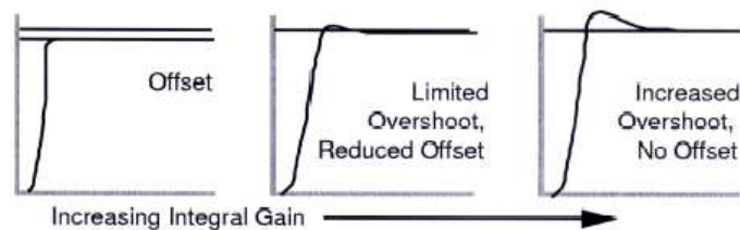
Figure 3.21: The effect of the integral coefficient on the signals
