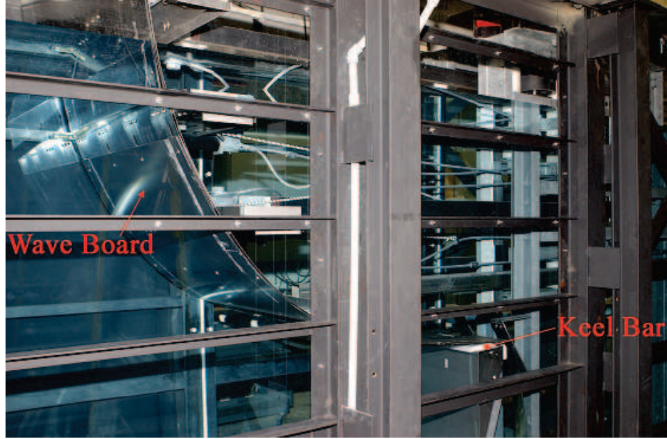
Figure 3.11: The 2D+T wave maker in a stationary fully extended state
