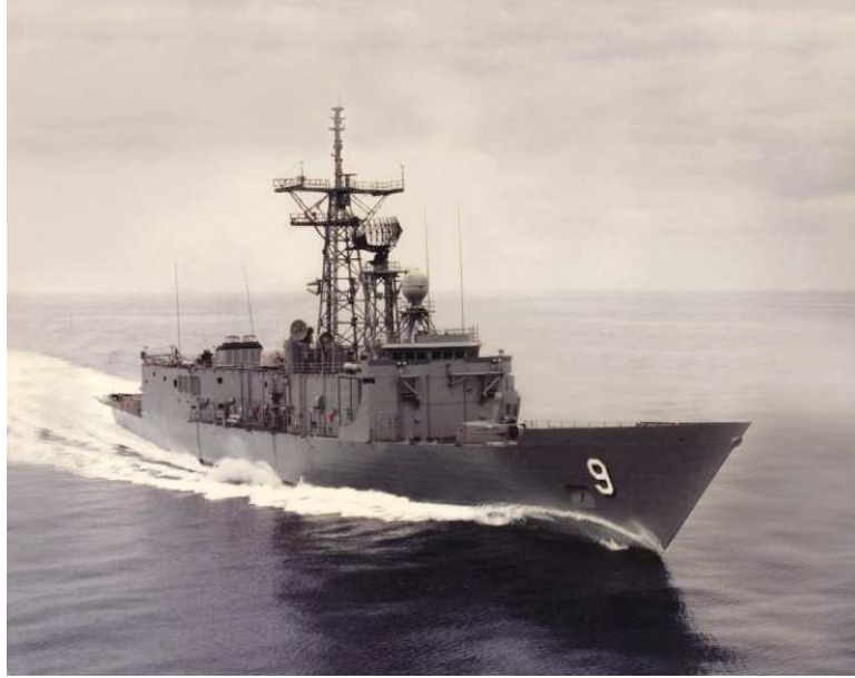
Figure 1.2: A photograph of a US Navy Frigate showing a plunging breaker forming from the bow.
