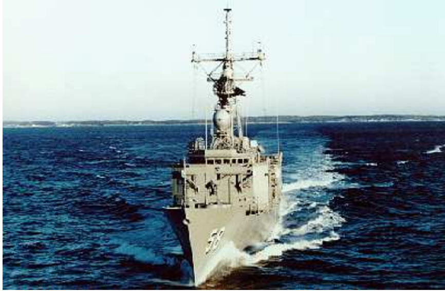
Figure 1.1: A photograph of a US Navy Frigate showing a strong plunging breaker formed in either side of the bow.
