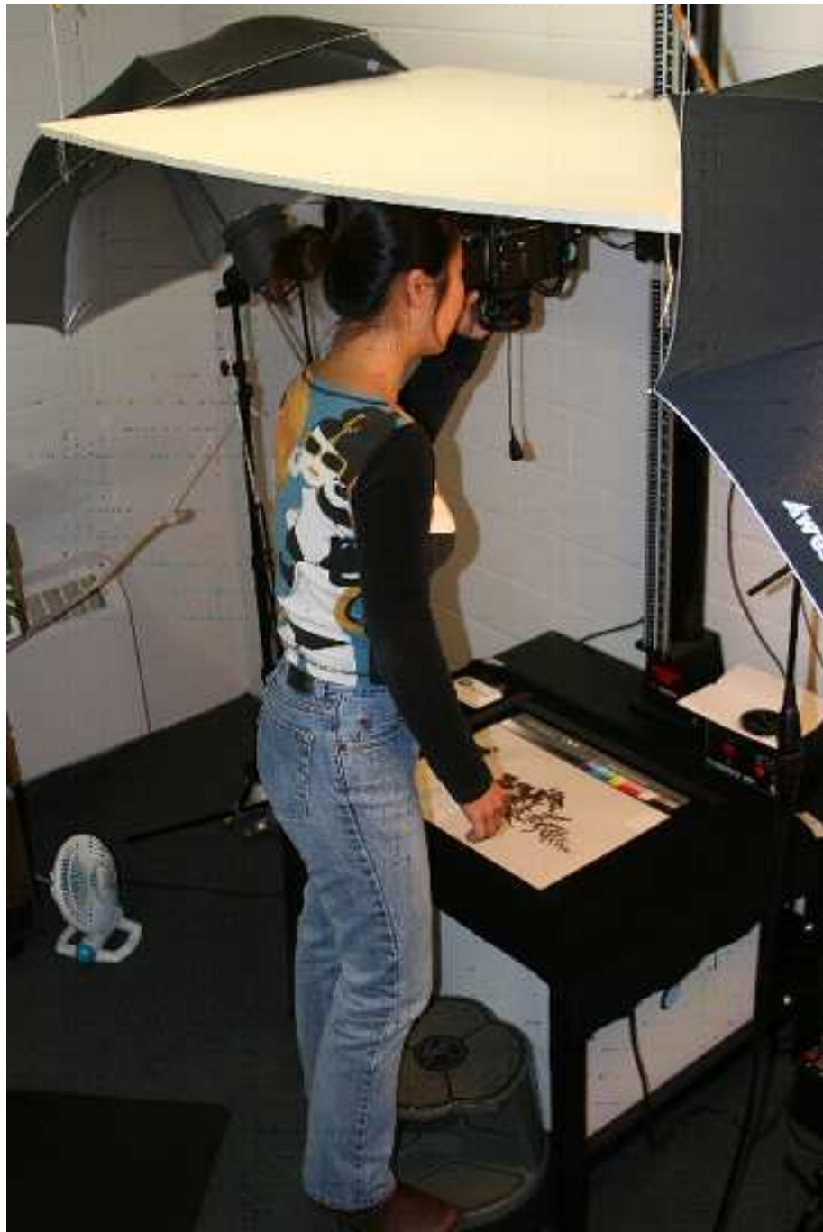
Figure 7.1: The present database has been photographed under controlled lighting conditions. One H20 back on Hasselblad 502 with 80mm lens has been used to get images of resolution 3600x5000 pixels
