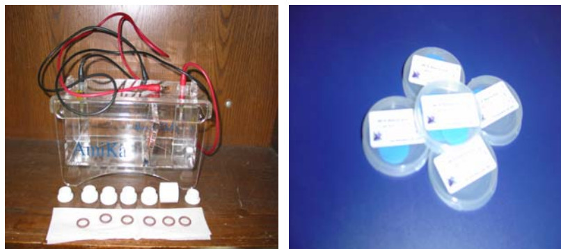
Figure 3-1 Photographs of the solution isoelectric focusing device used in our lab. Left: the electrophoresis tank (Amika Corp.), Teflon chambers and caps (multichamber Teflon dialyzer system, Amika Corp.) and 12-mm-i.d. O-rings (Scientific Instrument Services, Inc., Ringoes, NJ); Right: pH membranes 3-5-6.5-8-11 (ProteomeSystems, Inc., Woburn, MA)
