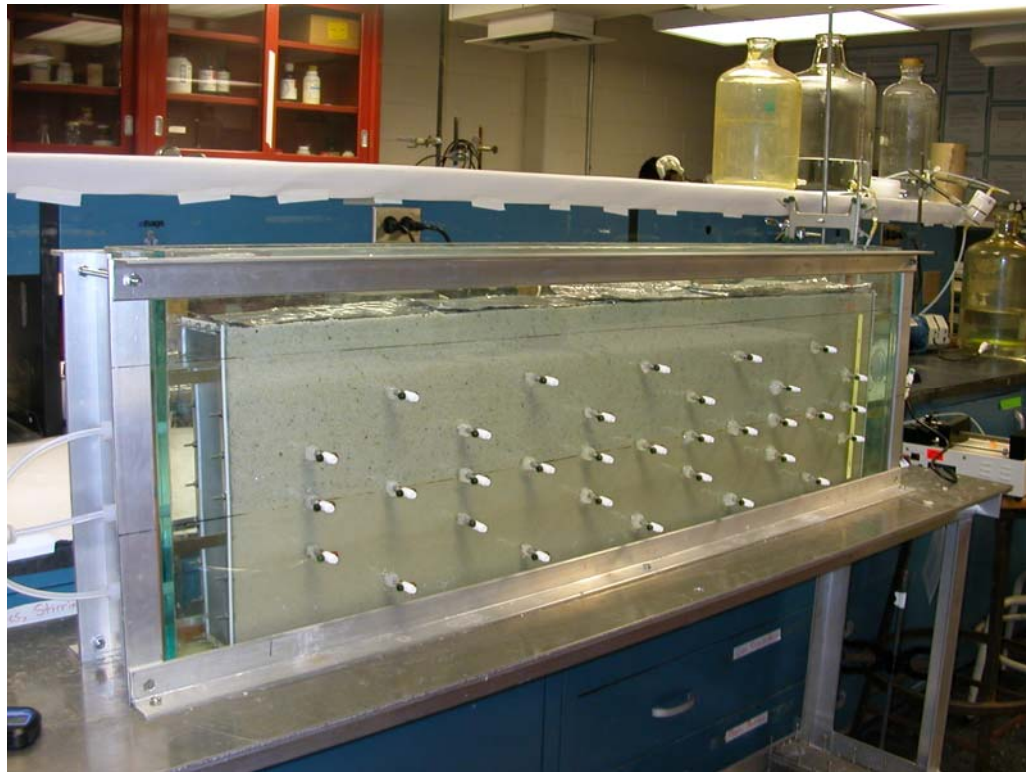
Figure 5.4 Glass ISFC with screens, sampling ports, and aluminum frame and cart.
