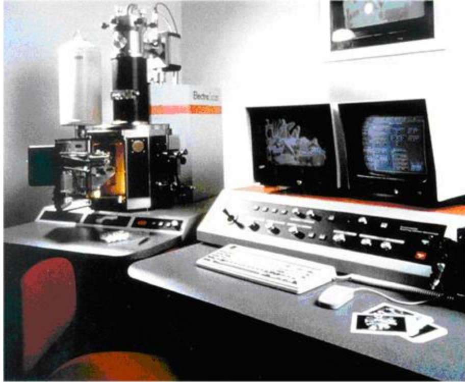
Figure 2.6 Picture of the E-SEM test apparatus
