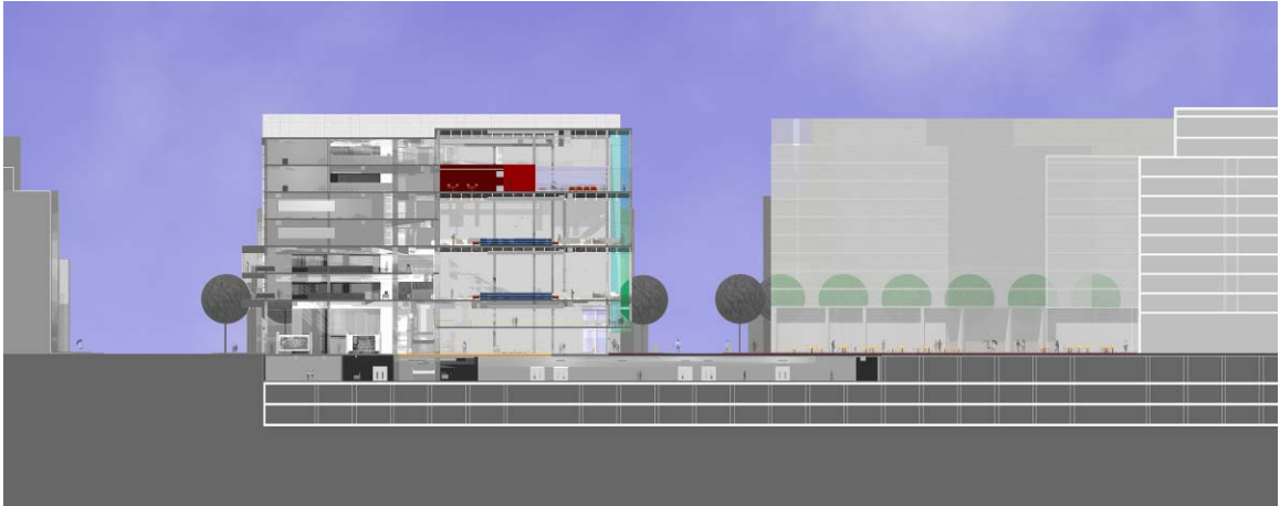
Figure 131-Site section showing the relationship between the major spaces, the plaza, and the context mixed-use building. The drawing also shows the relative heights of programmatic functions
