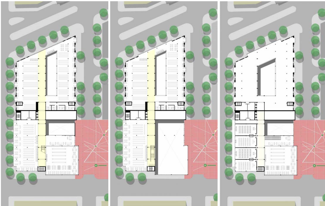
Figure 126-Stacks, stacks mezzanine, and classroom plans. These drawings show the relationship between voids, and the relationship between the stacks levels, and the office component
