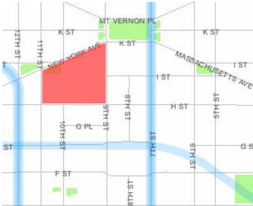
Figure 61-Diagram showing the Metro tunnel system around the site. There are no tunnels beneath the site, allowing for program below grade (DC Planning)
