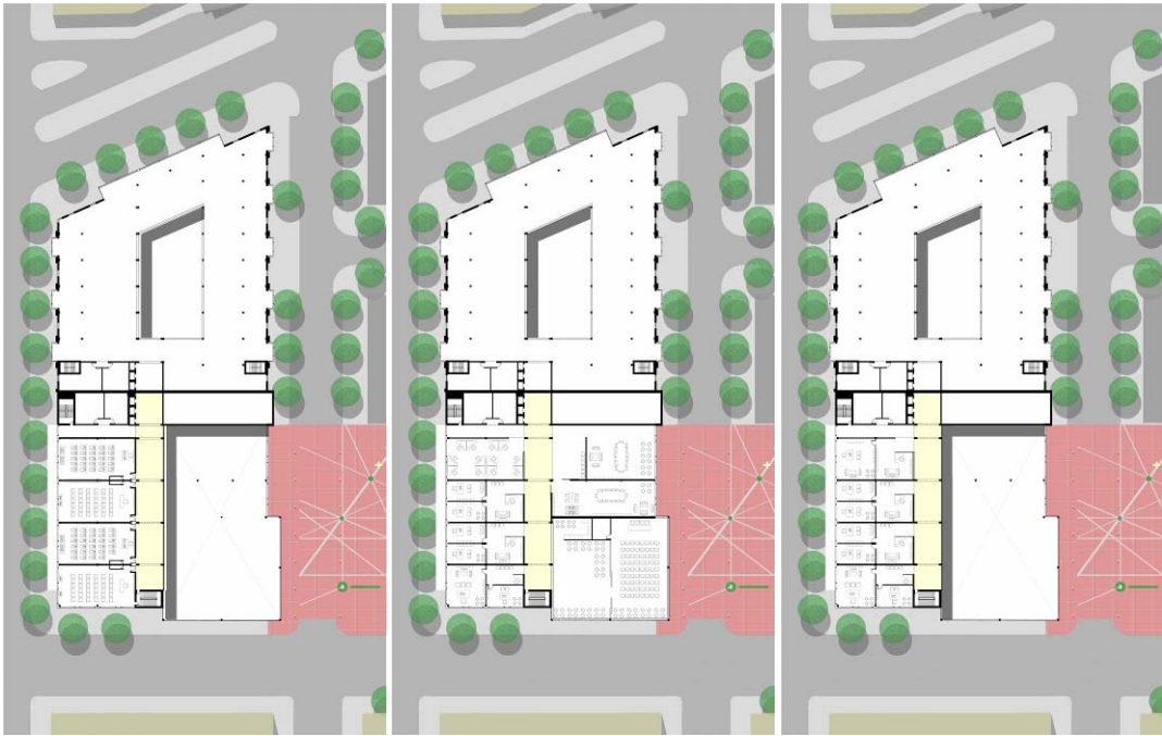
Figure 127-Classroom mezzanine, office and office mezzanine plans. These drawings further emphasize the horizontal stacking of the building, and the relative sizes of program pieces
