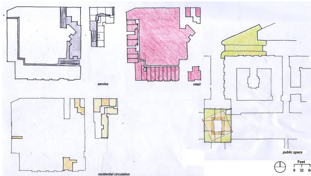
Figure 78-Diagrams showing the disposition of program, including service, retail, vertical residential circulation, and major public spaces
