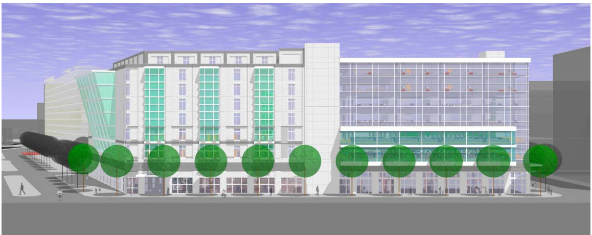
Figure 133-West elevation showing the difference between the north and west facades, and the level of transparency of the glass curtain wall
