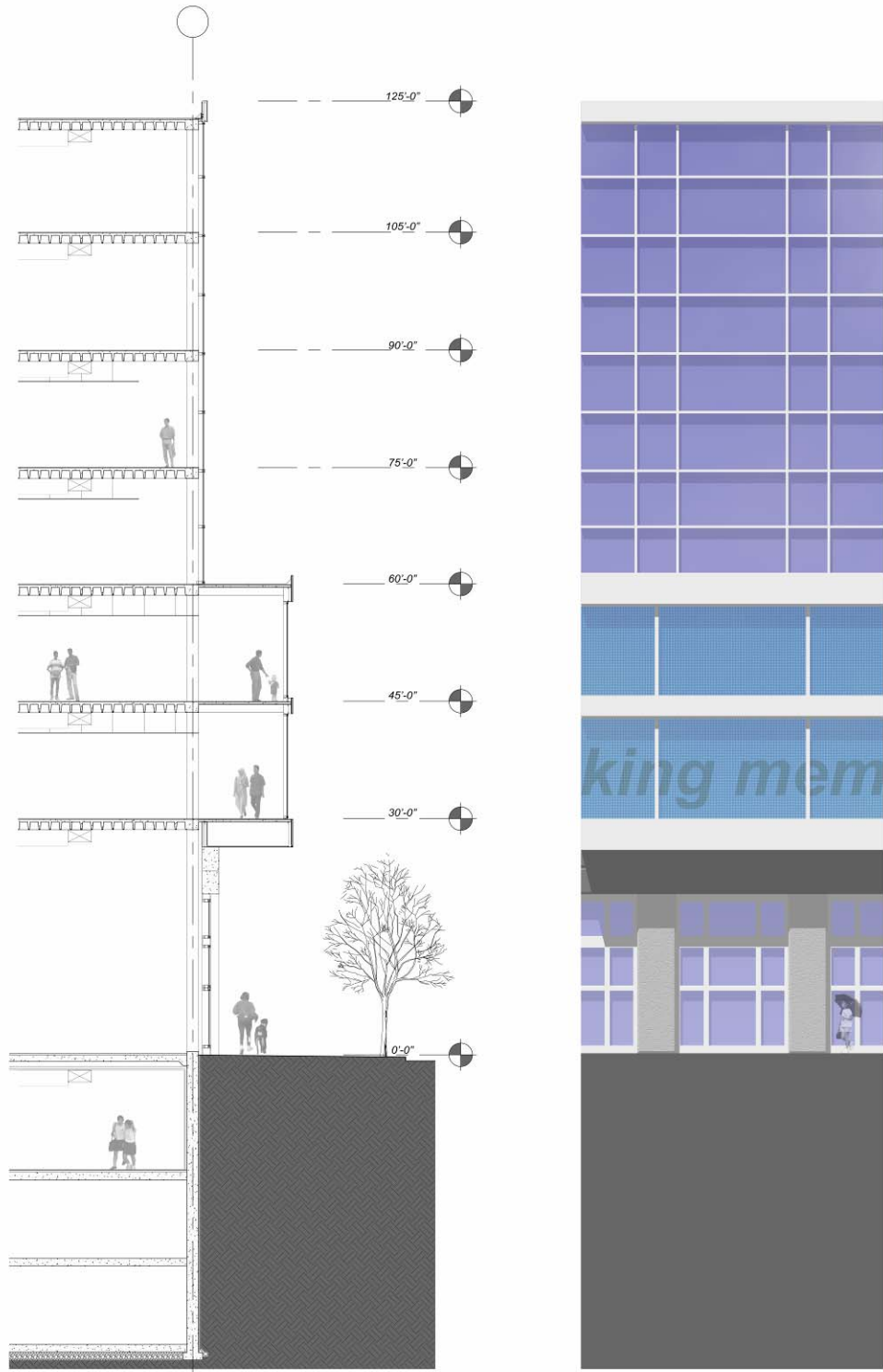
Figure 147-Wall section through western elevation, showing the three main parts of the facades, the glass curtain wall, the translucent glass in the reading rooms and stacks areas, and the ground level bay system
