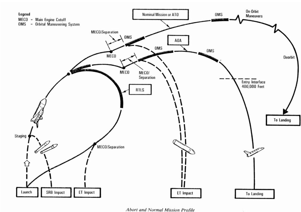
Figure 2.5 Shuttle Intact Abort Modes [8]
