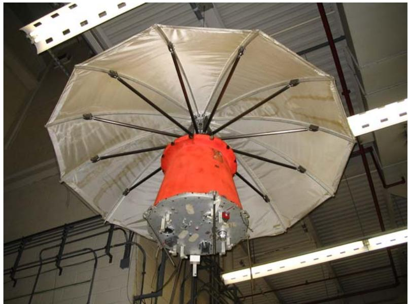
**Figure 2.4 Parashield, lightweight, low beta reentry design**
