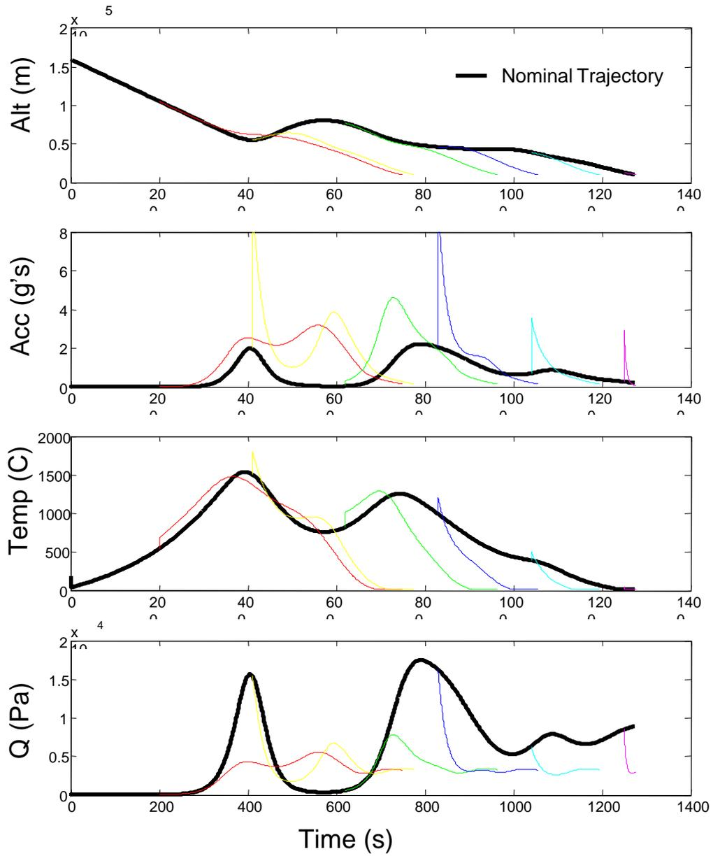
**Figure 5.7 Sampling of Simulation Trajectory Results Evenly Space Over Nominal Trajectory for Optimal Lifeboat with Design Characteristics of  $\beta=650 \text{ kg/m}^2$ ,  $L/D = .2$  and Heat Shield Radius=2.8 m.**
