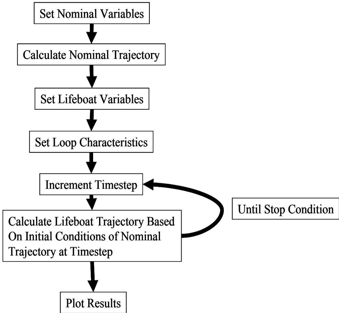
Figure 4.4 Algorithm used in computer simulation
