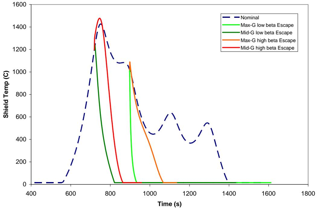
Figure 5.3 Spreadsheet Simulation Results, Outer Shield Temperature vs. Time
