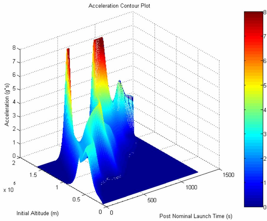
**Figure 5.9 Three Dimensional Mesh Plot of Acceleration vs Altitude and Time with Maximum Acceleration set to 8 g's**
