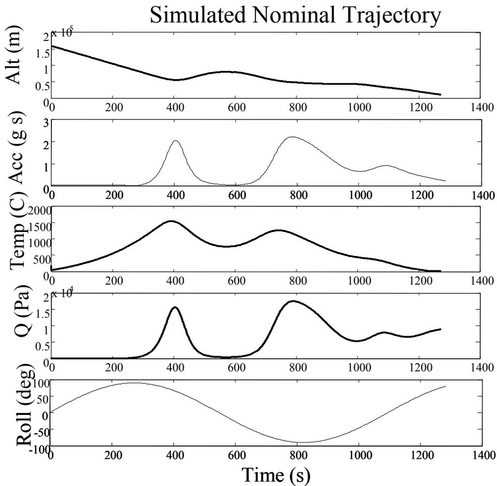
**Figure 4.1 Simulated Nominal Trajectory**
