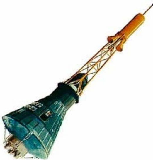
**Figure 2.2 Mercury Capsule with Launch Escape Tower**
