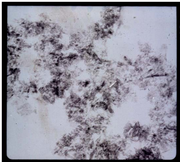
Figure 2.4 Microgram of Pd crystallites on a \gamma - \text{Al}_2\text{O}_3 support
