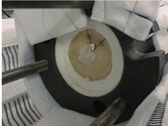
Figure 2-6: Temperature measurement of a ZnSe window with a K-Type thermocouple.
