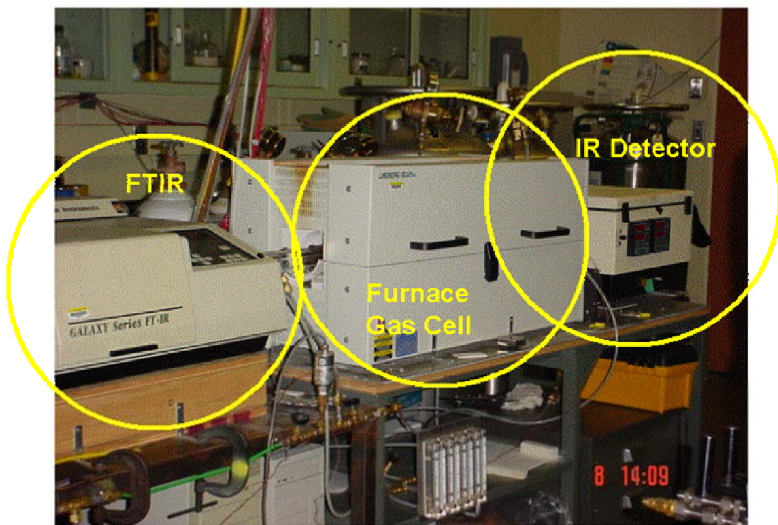
Figure 2-4: Picture of high temperature FTIR test rig.
