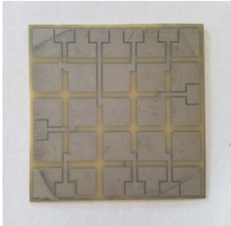
Figure 27: Full 5x5 etched piezoelectric prototype grid
