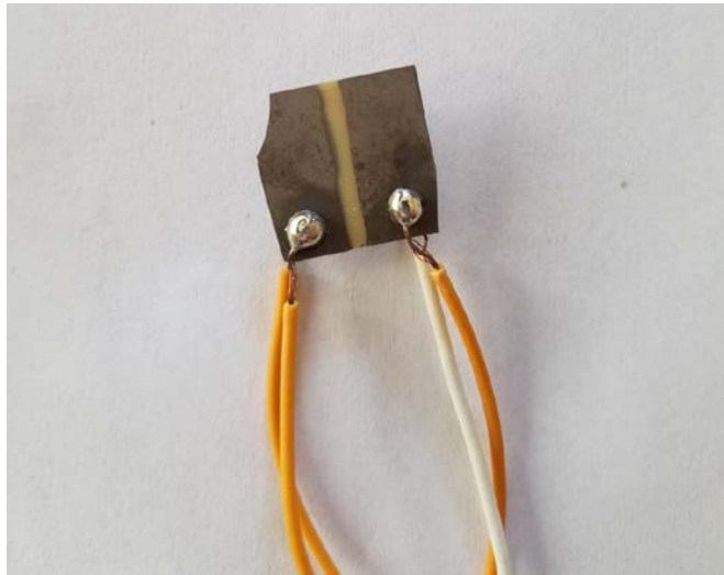
Figure 24: Two part etched piezoelectric element for initial testing/proof of concept
