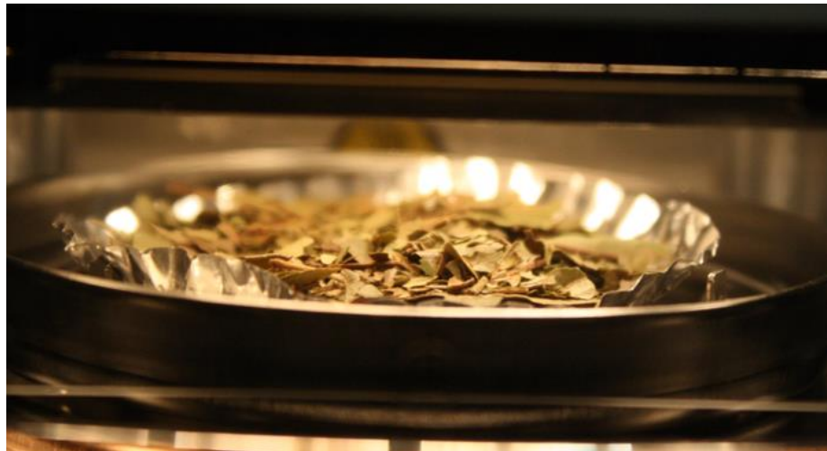
Figure 7: (top) The moisture content analyzer with the lid open showing the sample tray. (bottom) Northern bayberry being tested for MC level via the halogen heating lamp. Note that the leaves were crushed prior testing
