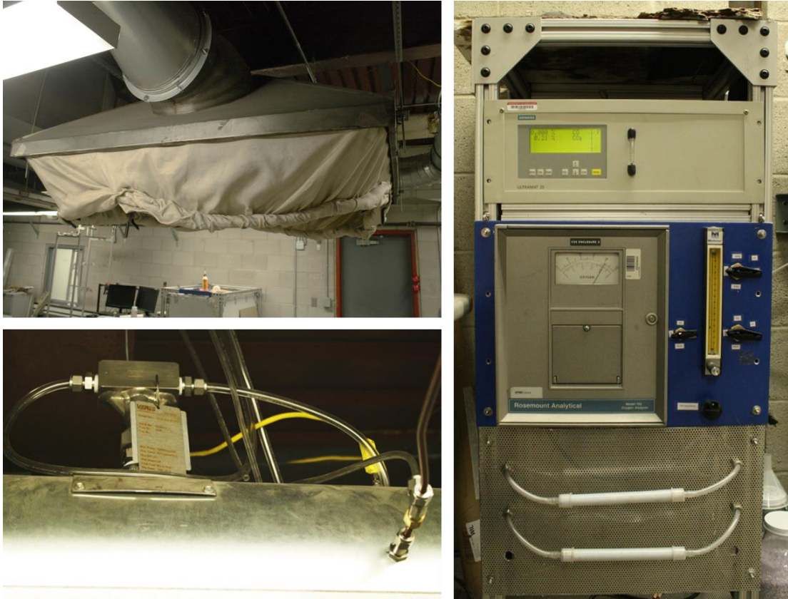
Figure 9: (Top left) Exhaust hood with containment curtain rolled up. (Bottom left) Pitot tube, thermocouple, H 2 O analyzer, and gas sampling ports. (Right) Gas analysis rack, with CO/CO 2 sensor above and O 2 below.
