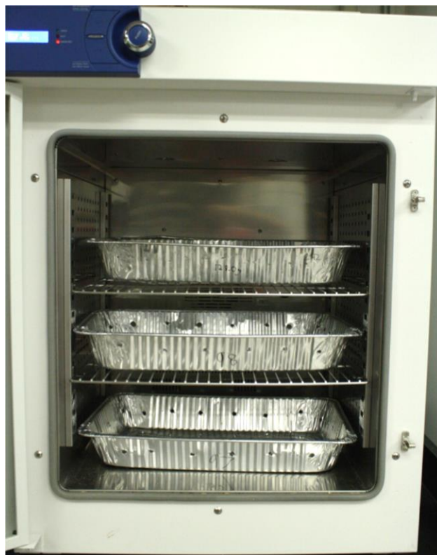
Figure 6: VWR drying oven with door open. Three aluminum trays with holes drilled for enhanced air circulation could be placed in the oven at one time
