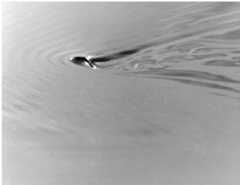
Figure 3.6: Below-water view of the jet impact site for no air entrainment conditions. V_j = 303 \text{ cm/s} , D_j = 0.6 \text{ cm} , V_t = 31.8 \text{ cm/s}
