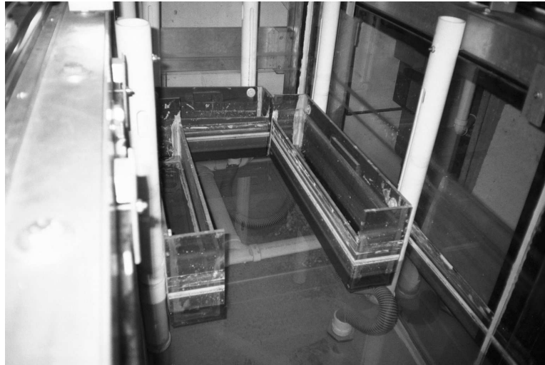
Figure 4.9: Picture of the three water skimmers at one end of the new facility. The skimmers remove the contaminants from the water free surface and send them to a filter
