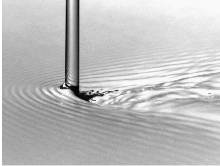
Figure 3.7: Above-water view of the jet impact site for incipient entrainment conditions. V_j = 303 \text{ cm/s} , D_j = 0.6 \text{ cm} , V_t = 38.51 \text{ cm/s}
