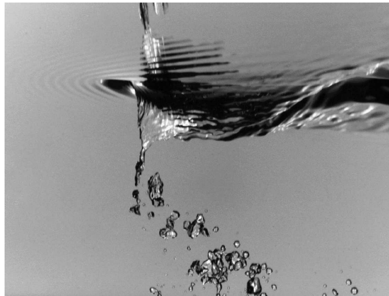
Figure 3.10: Below-water view of the jet impact site for intermittent entrainment conditions. V_j = 303 \text{ cm/s} , D_j = 0.6 \text{ cm} , V_t = 44.5 \text{ cm/s}
