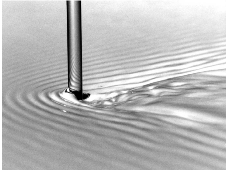
Figure 3.5: Above-water view of the jet impact site for no air entrainment conditions. V_j = 303 \text{ cm/s} , D_j = 0.6 \text{ cm} , V_t = 31.8 \text{ cm/s}
