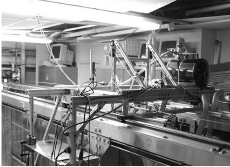
Figure 4.7: Picture of the new instrument carriage. In the image are visible several of the described elements such as the supporting trays for the camera and computer on a side of the tank, the structure that holds the jet nozzle, the long aluminum structures that hold the carriage rails, the bearing systems and the compressed-air reservoir for the jet cutter device (described in later sections).
