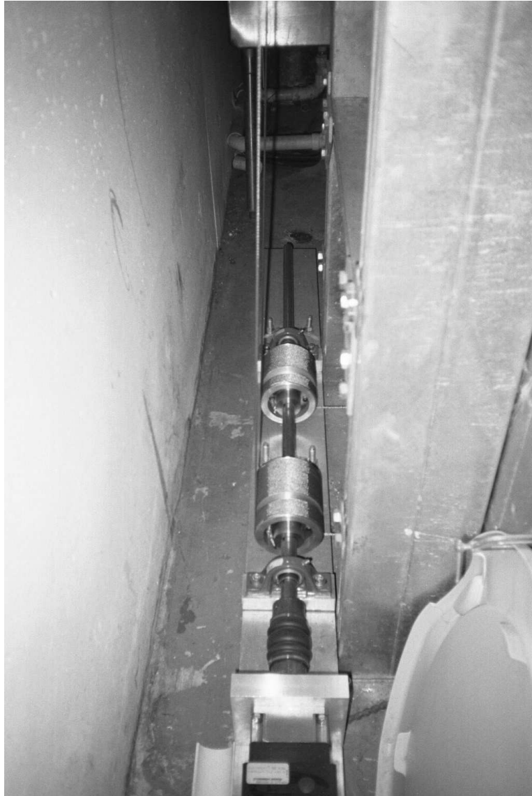
Figure 4.6: Picture of the aluminium drums, shaft, universal joint and steel towing cable
