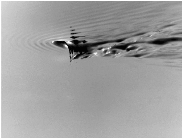
Figure 3.8: Below-water view of the jet impact site for incipient entrainment conditions. V_j = 303 \text{ cm/s} , D_j = 0.6 \text{ cm} , V_t = 38.51 \text{ cm/s}
