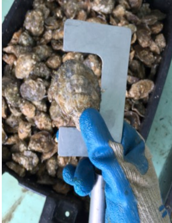
Figure 5. Custom manufactured grading tool used to grade oysters to at least 63.5 mm before deployment, to ensure uniformity of initial samples.
