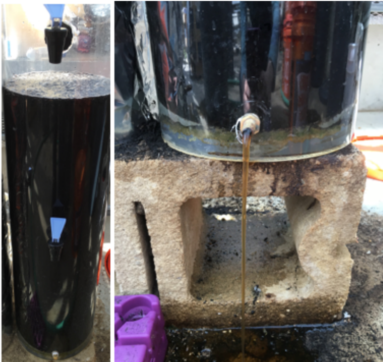
Figure 4. Compost washing procedure: compost soaking in tap water (left) and draining off of effluent (right)
