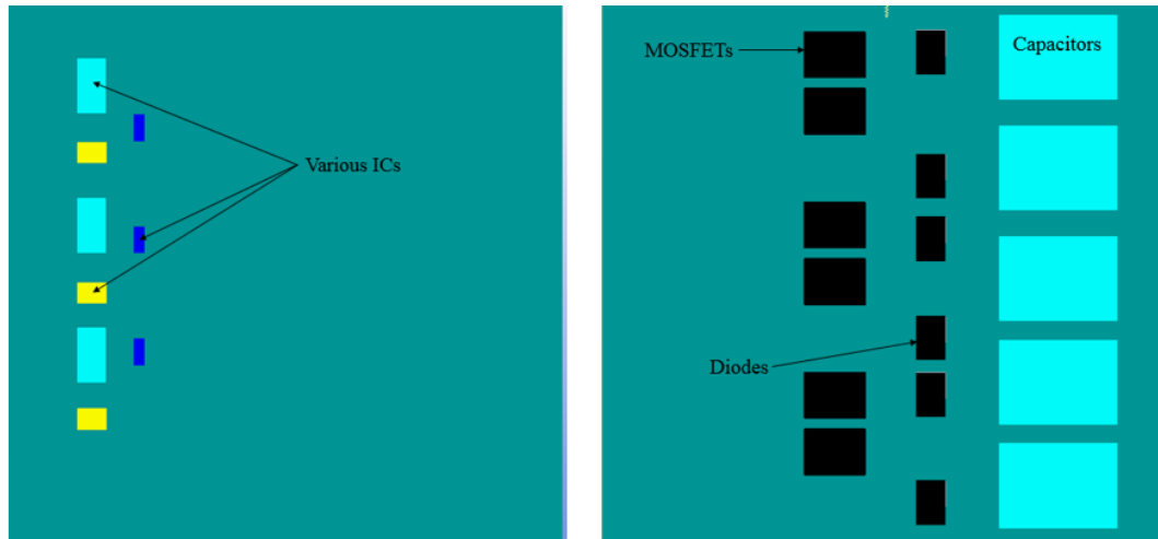
Figure 3-3: Top view (left) and bottom view (right) of PFC PCB in Icepak
