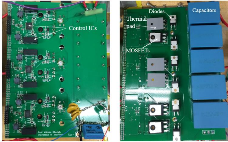
Figure 1-4: Top side (left) and bottom side (right) of PFC board
