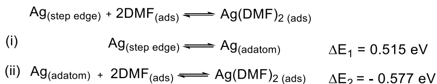
Scheme 4.3. The formation of \text{Ag}(\text{DMF})_2 and two underlying reaction steps.
