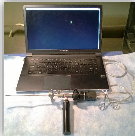
Figure 2. Benchtop laparoscopy setup for use with chemically anesthetized largemouth bass Micropterus salmoides , computer used for viewing and blocks for holding fish.
