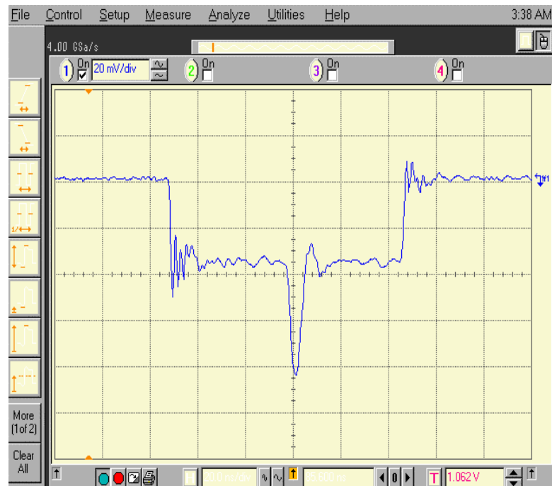
Figure 1.4 Beam current of the photo and thermionic emission electron beam measured by Bergoz current transformer
