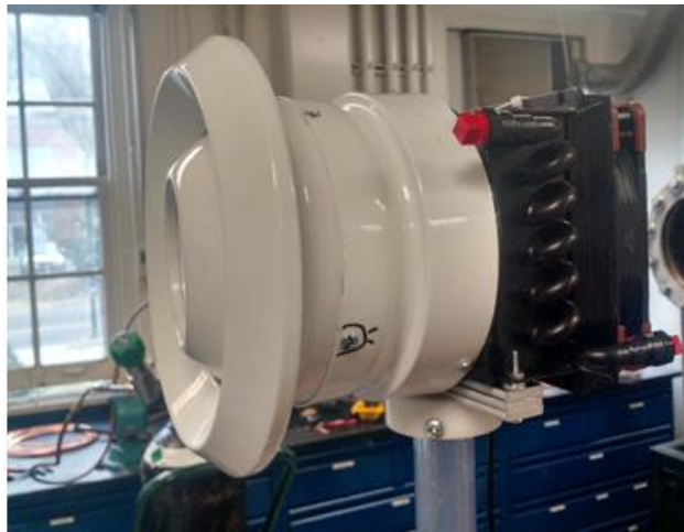
Figure 45: Nozzle-evaporator-fan assembly in the prototype
