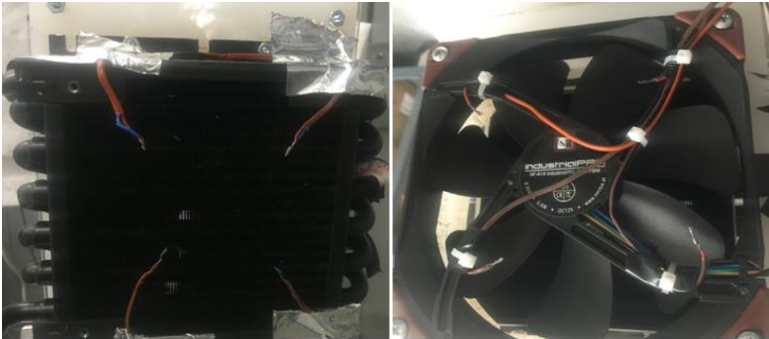
Figure 18: Airside thermocouple locations
