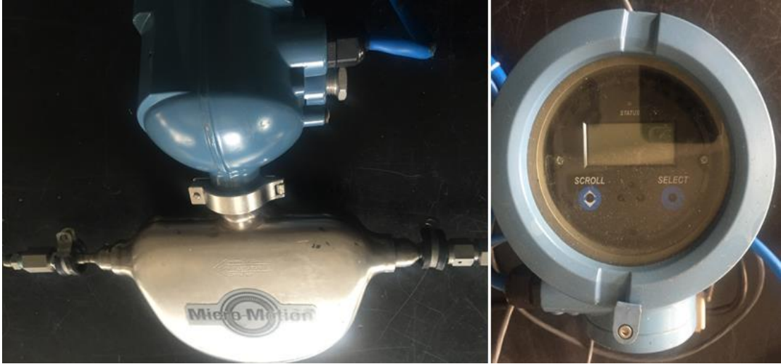
Figure 21: Mass flow meter and the transmitter
