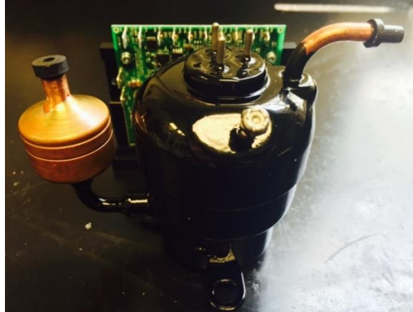
Figure 6: Aspen compressor and high capacity drive
