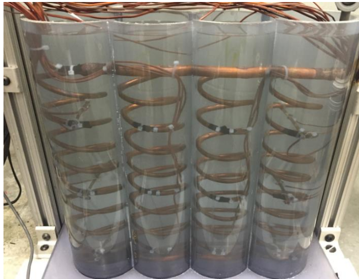
Figure 26: Liquid phase PCM inside condenser container
