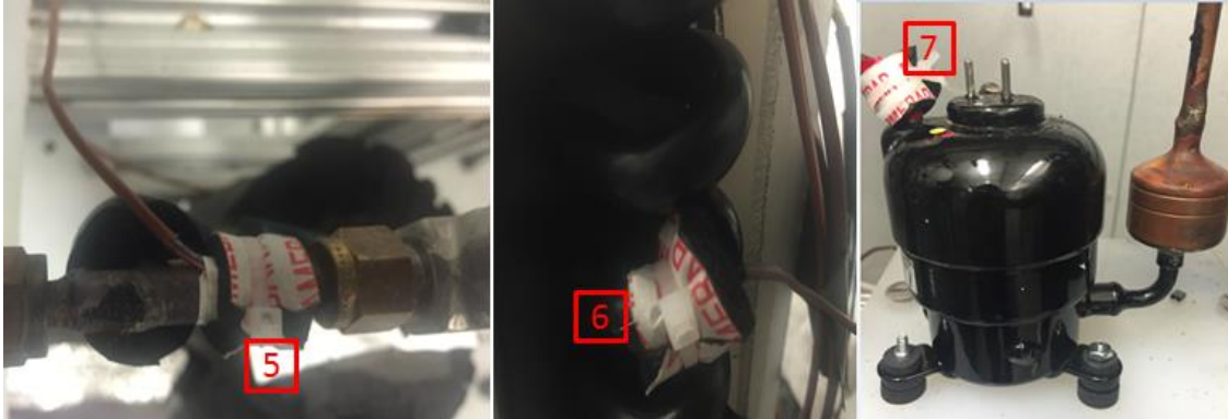
Figure 17: Refrigerant side surface thermocouple locations
