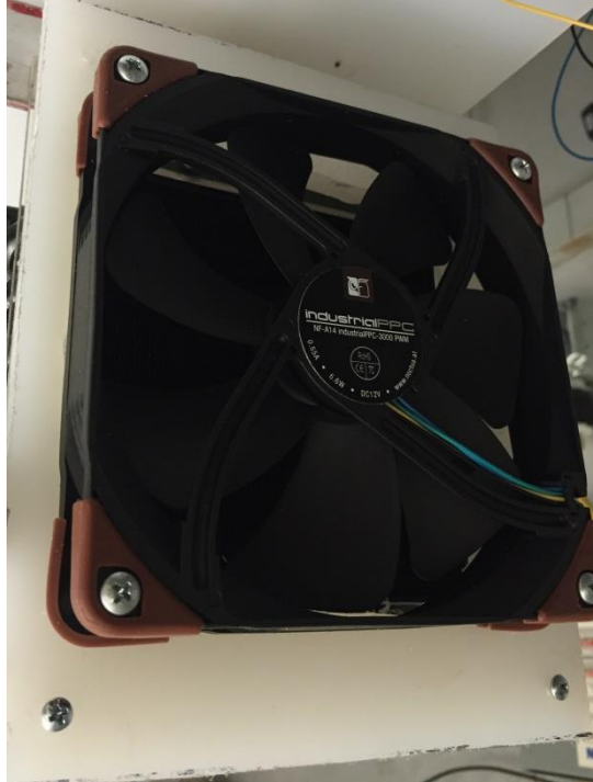
Figure 8: Noctua NF-A14 PWM cooling fan
