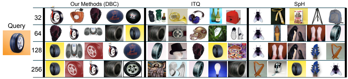
FIGURE 3.7: This figure qualitatively compares the quality of retrieved images by our method comparing to that of ITQ and SpH. Each row corresponds to the top five images returned by three different methods: ours, ITQ and spectral hashing. This retrieval is done by first projecting the query image to the space of binary codes and then running KNN in that space. Notice how, even with relatively short codes(32 bits), our method recovers round objects. Our method is consistent in terms of returned images as we increase the code size. With 256 dimensional code our method returns 5 correct images.
