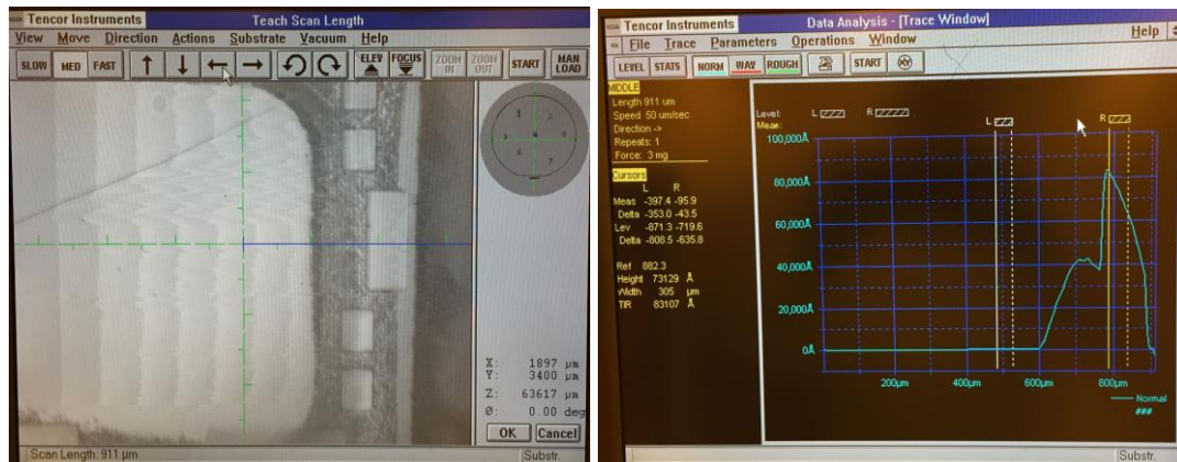
Figure B.2. (Left) Blue line is the scan direction on a developed sample using stamp method. (Right) The profile of the sample showing an edge bead that cannot be developed.
