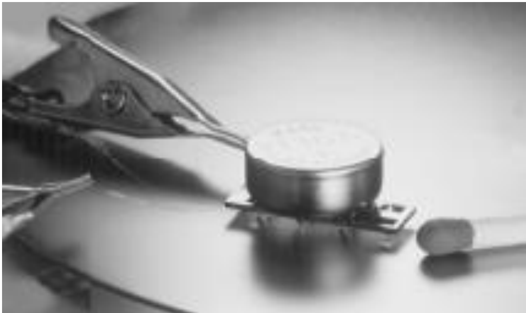
Figure 1.8. Walking silicon robot carries a load. Power and control signal are provided externally through the bond wires [26]. A match on the right is used to indicate the size. Figure taken directly from the reference [26].
