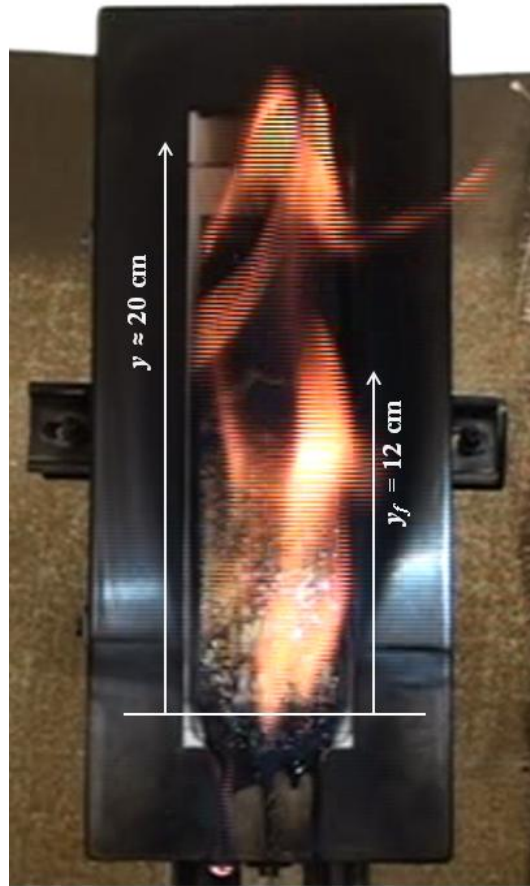
Figure 62. Flame height comparison during upward flame spread over PMMA EXT
