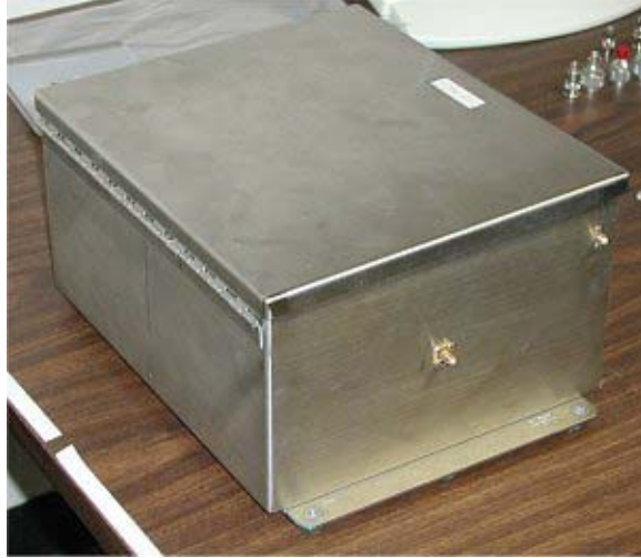
Figure 3.4 Stainless steel enclosure (cavity) with SMA connectors at the port locations.
