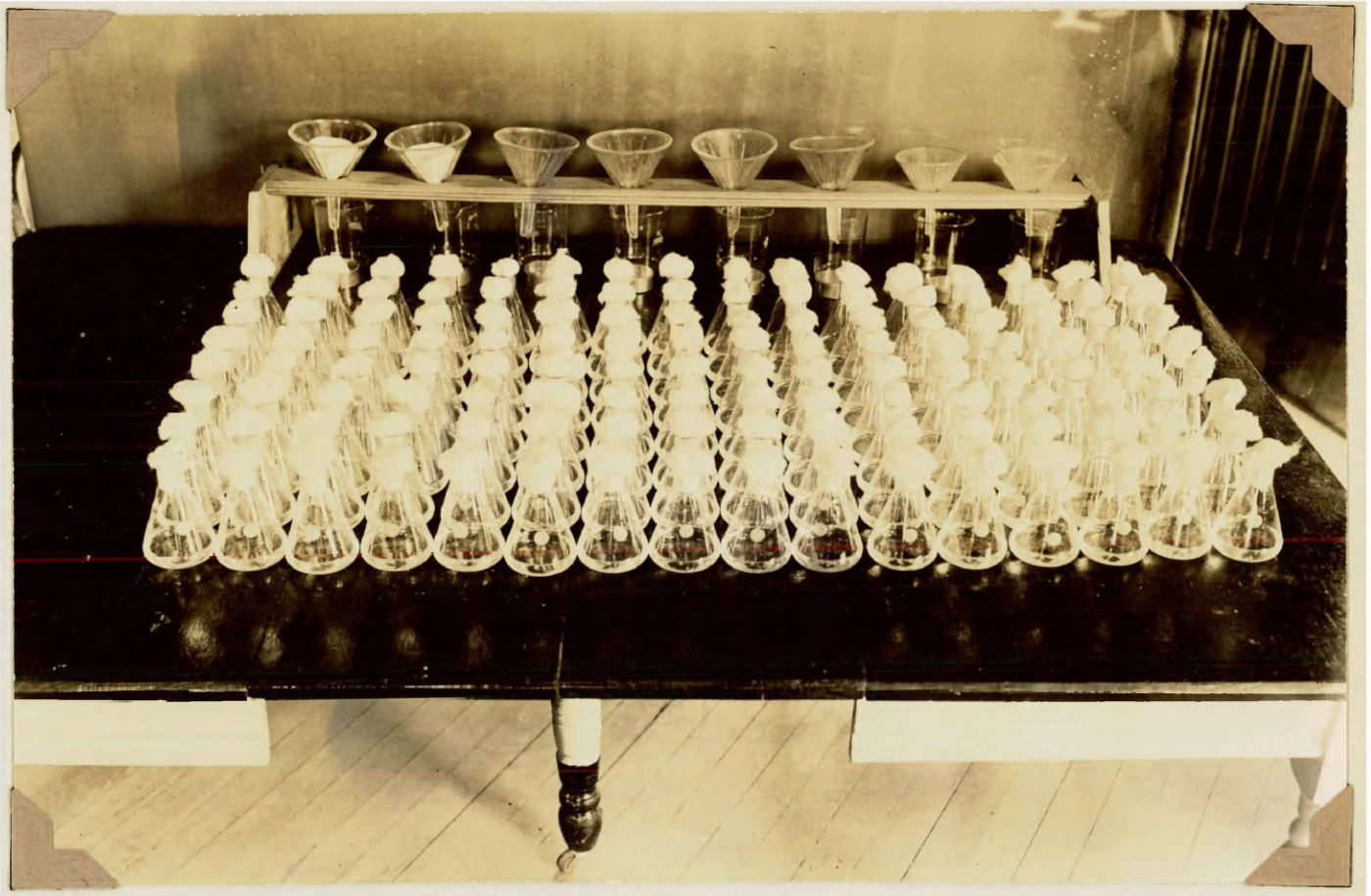
Fig. 1. A series of the 125 cc. Pyrex Erlenmeyer culture flasks containing 40 cc. of the nutrient solution. (Just after inoculation). In the background are the glass funnels, filter paper and weighing cups used in the dry weight determinations of the mycelium.
