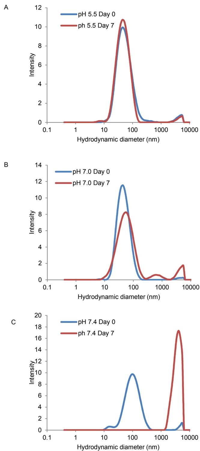
**Figure S2.** Hydrodynamic diameter intensity distributions of PBNPs in varied pH. PBNP sizes were quantified by dynamic light scattering (DLS) over 7 days (Day 0: blue, Day 7: red) at pH A) 5.5, B) 7.0, and C) 7.4, illustrating stability at mildly acidic/neutral pHs that mimic tumor interstitia and instability at mildly alkaline pHs (7.4) mimicking the lymph and blood.
