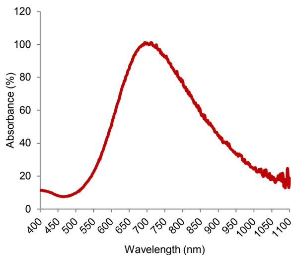
**Figure S1.** Vis-NIR spectrum of PBNPs. PBNPs were analyzed using the VISIONlite software on the Genesys 10S spectrophotometer (Thermo Scientific, Waltham, MA).
