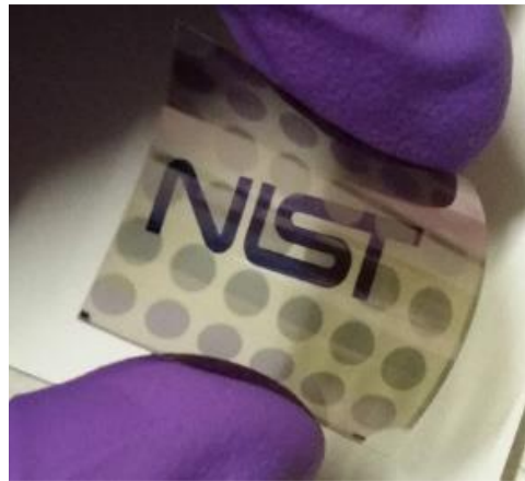
Fig. 4.16 The fabricated device exhibiting flexibility and transparency
