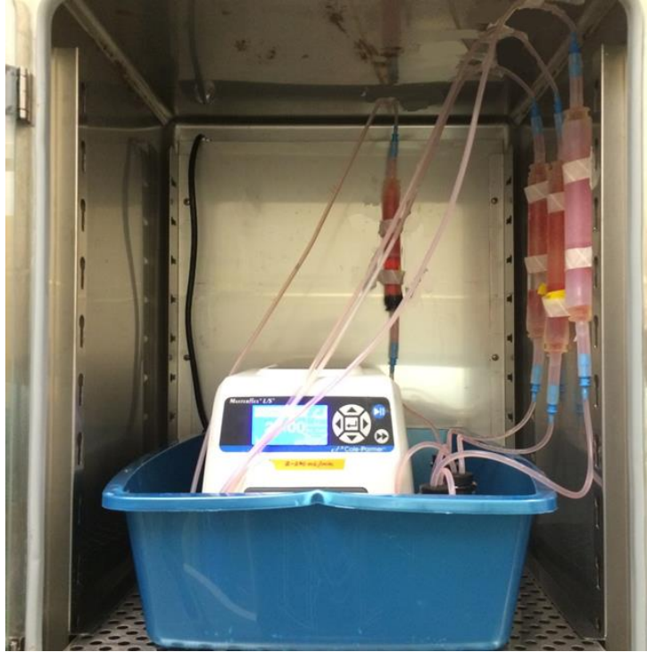
Figure 9: Bioreactor Setup Featuring 4 Experimental Groups in Parallel
