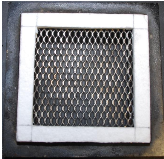
Figure 13. Sample holder with aluminum mesh and Kaowool.
