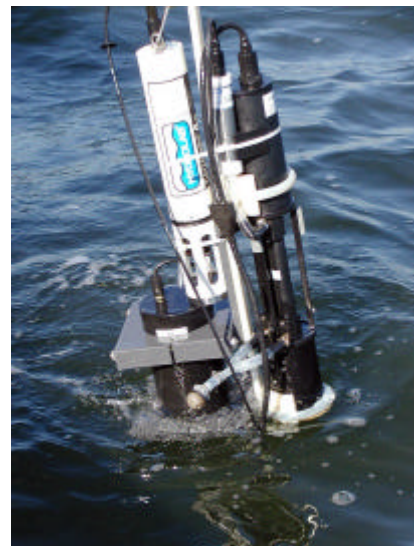
Figure 2.2-2: The AC9 instrument (far right in the picture), the Hydrolab (white instrument in the middle) and the ECO-VSF instrument (far left) that were used during one of the cruises in the Chesapeake Bay.
