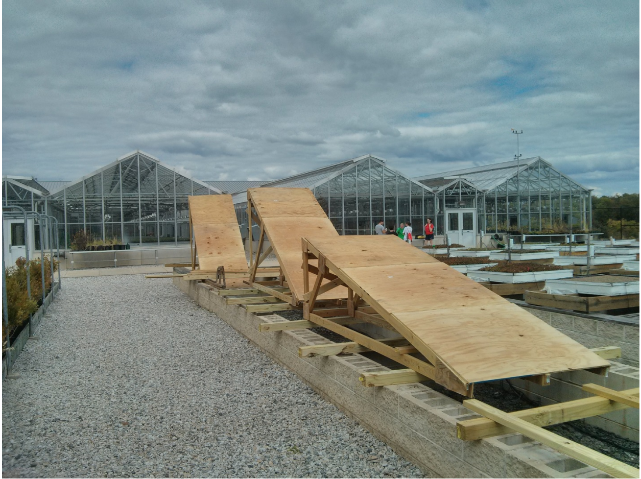
Figure 33. Overview of 15, 30, and 45 degree modules taken in Sep. 2012 (Courtesy of Ben Borchers)
