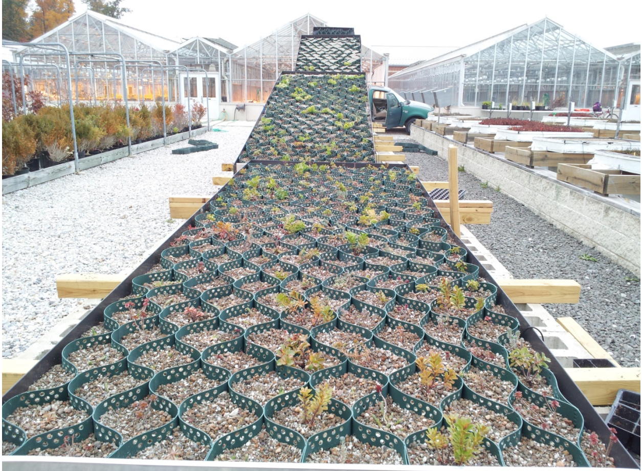
Figure 35. Overview of control, 15, and 30 degree modules after filling with substrate and planting. Taken in Oct. 2013 (Courtesy of Ben Borchers)
