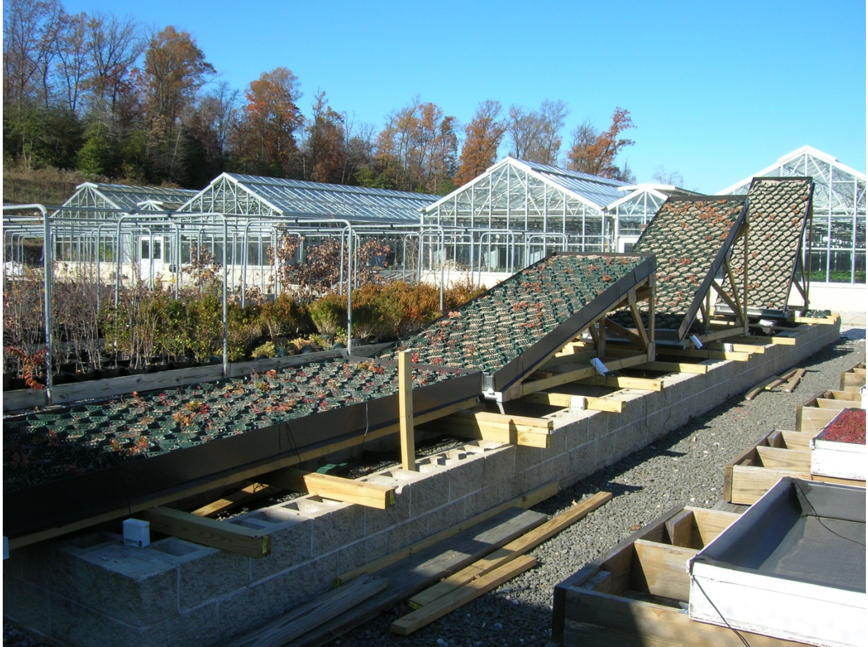
Figure 36. Overview of control, 15, 30, and 45 degree modules taken in Oct. 2013 (Courtesy of Ben Borchers)
