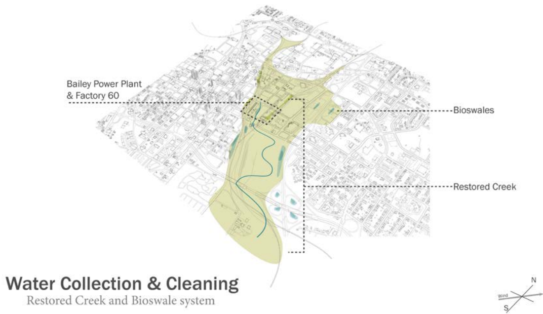
Figure 36: Bioswales collect and clean storm water runoff before it enters the creek. (Source: Author)
