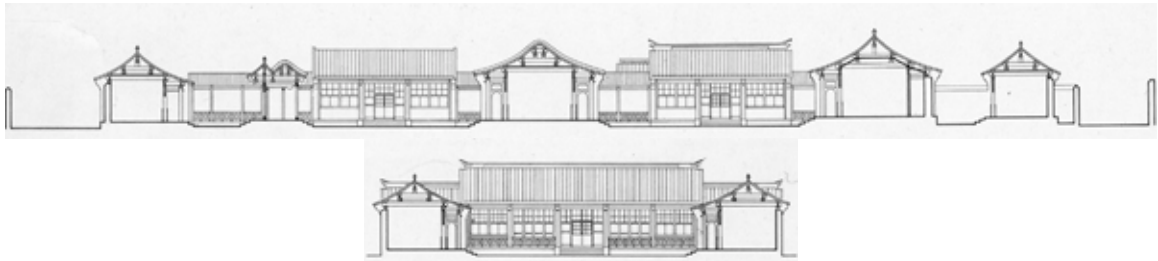
Figure 32: Longitudinal Section. 15 This section is cut along the main axis of the house, through the entry court and the two interior courtyards.
