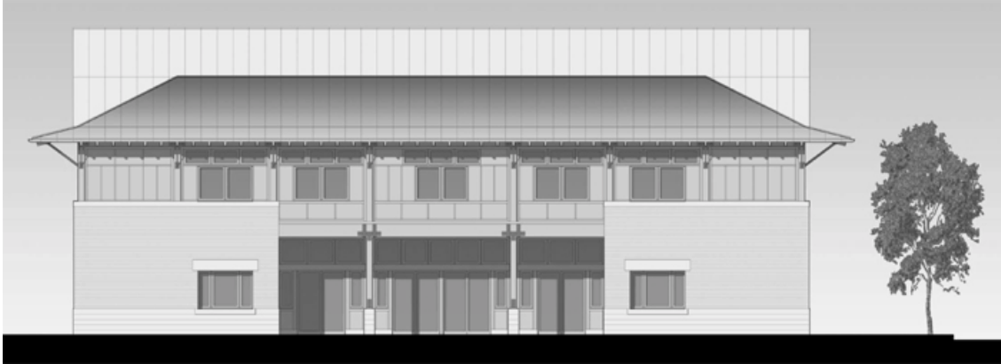
Figure 86: H St. Elevation. The entrance to the school is opened and set back, in order to create a shallow recess to welcome people.
