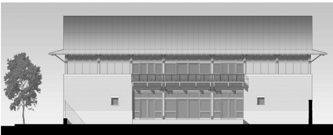
Figure 89: Garden Elevation. A balcony extends over the porch providing protection from the elements.
