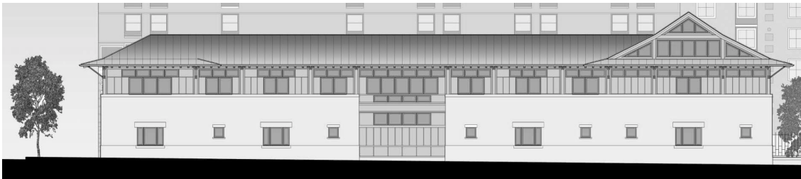
Figure 87: 6 th St. Elevation. The shape of the roof changes over the Training Hall, reflecting its importance.
