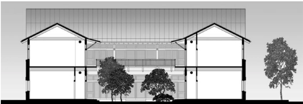
Figure 70: Cross Section through School and Courtyard. The school is organized around two courtyards. All programmed spaces have immediate adjacency to these exterior spaces, and on the second floor, an exterior balcony runs the perimeter of the courtyard.
