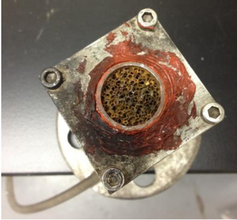
Figure 4-3 Top View of Cooling Device around Cold Heat Exchanger
