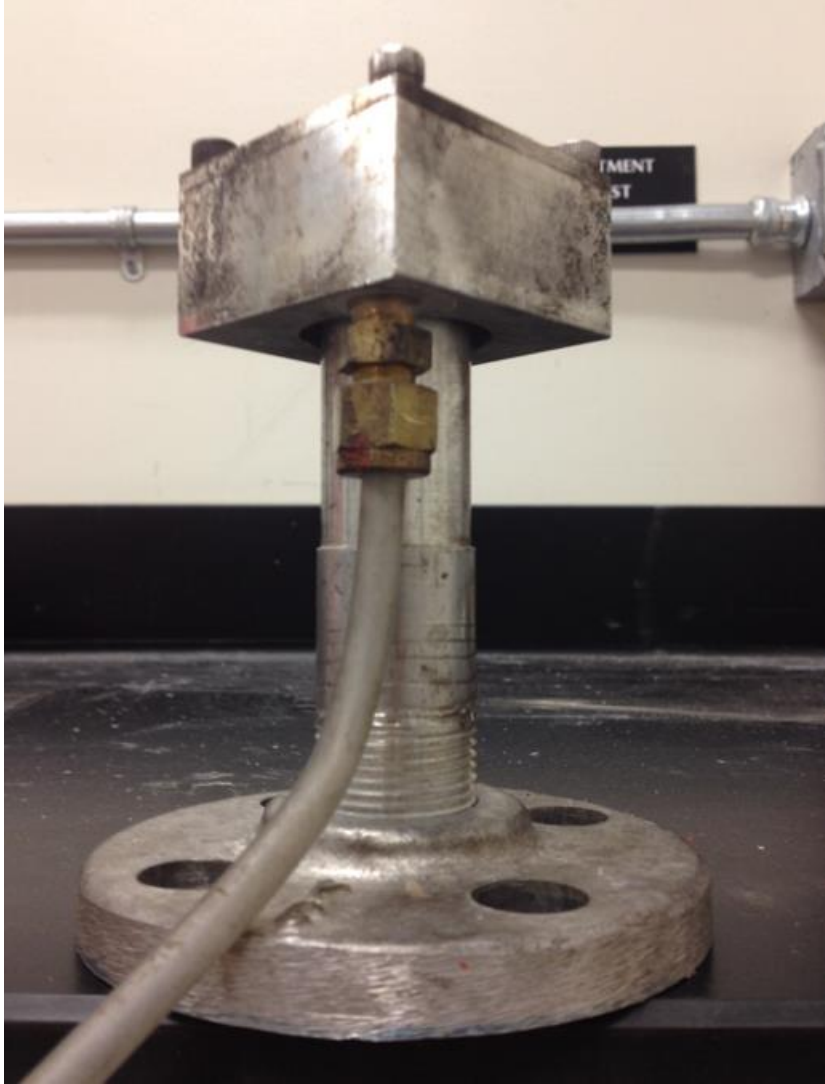
Figure 4-2 Side View of Resonator Tube with Water Cooling Device
