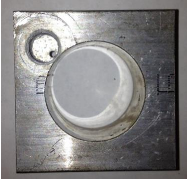
Figure 4-7 Bottom View of Bottom Piece of Cooling Device Showing Water Connection and Water Hole
