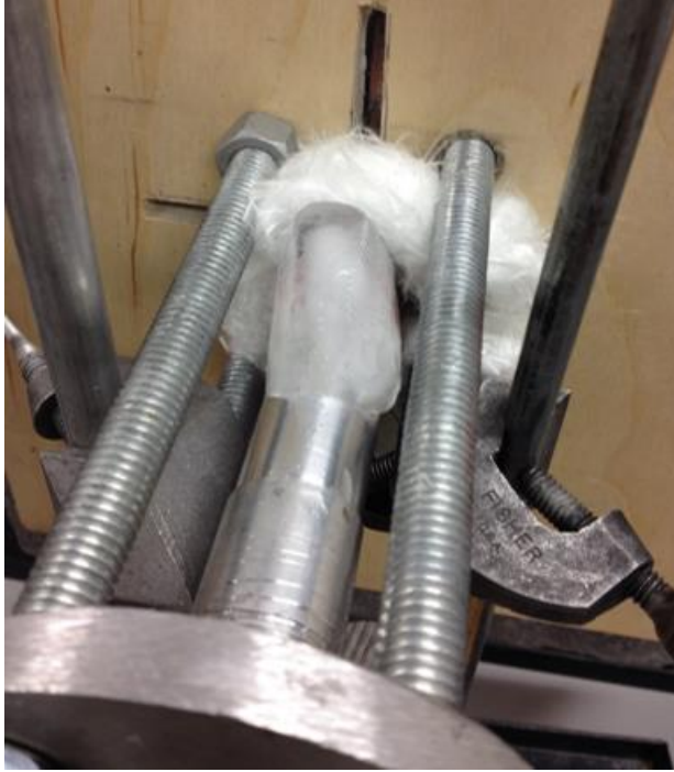
Figure 3-7 Insulation and Ice Cooling for Thermoacoustic Device during Radiant Panel Tests
