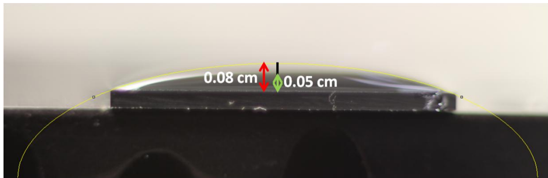
Figure 6-10. Fitting of the droplet surface to an arc to verify the gravity effect.
