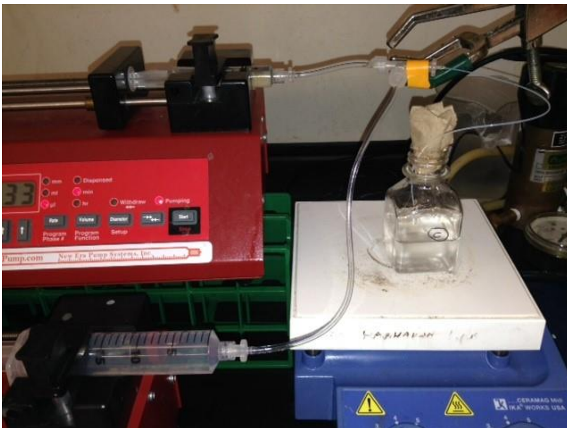
Figure A1. Microfluidic tubing device setup for the generation of chitosan microbeads. The 5 mL syringe (top) is loaded with the chitosan solution and the 20 mL syringe (bottom) is loaded with the oil solution. The collection vial, placed at the center of the stir plate, contains the cross-linking solution, which turns turbid when the glutaraldehyde is dispersed in the oil. The tip of the PTFE tubing is submerged in the GA solution, but should be held close to the surface of the liquid (i.e. it should not be in contact with the bottom or the walls of the vial).
