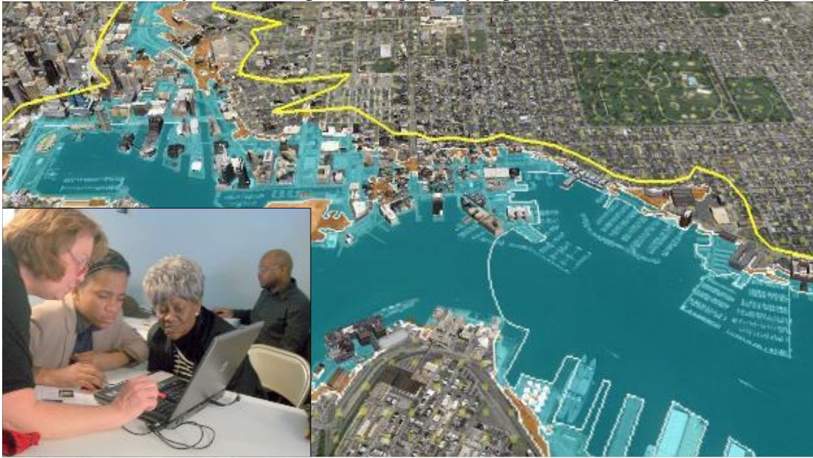
Figure 6: Stakeholder-built computer-assisted decision support system method showing anticipated future flood risk - Google Earth™ image with the Federal Emergency Management Agency 1% annual flood risk area shown in the blue layer. The yellow line was added by the stakeholder using the Google Earth™ drawing tool guided by Google Earth™ elevation data. This represented anticipated flood risk within the next 50 years. The area below the yellow line represented property expected to experience flooding.
