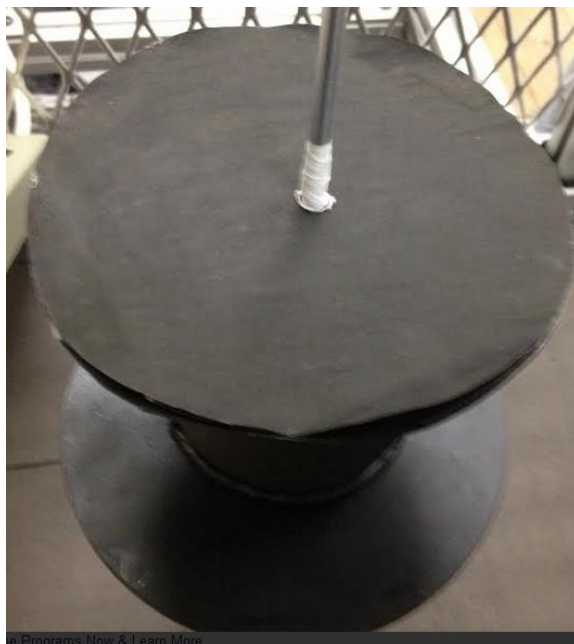
Figure 2.5. White tape and paper shell used to help track lateral displacements.
