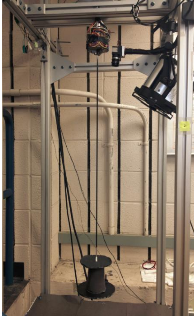
Figure 2.1. Experimental arrangement used to study the dynamics of a drill-string section. The rotor is at the bottom and a chuck is used at the top.
