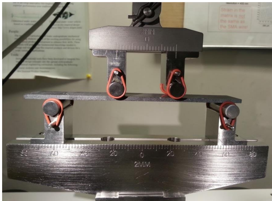
Figure 3.6: The Carbon fiber laminate specimen in the 4 point bend fixture testing the modulus in longitudinal direction
