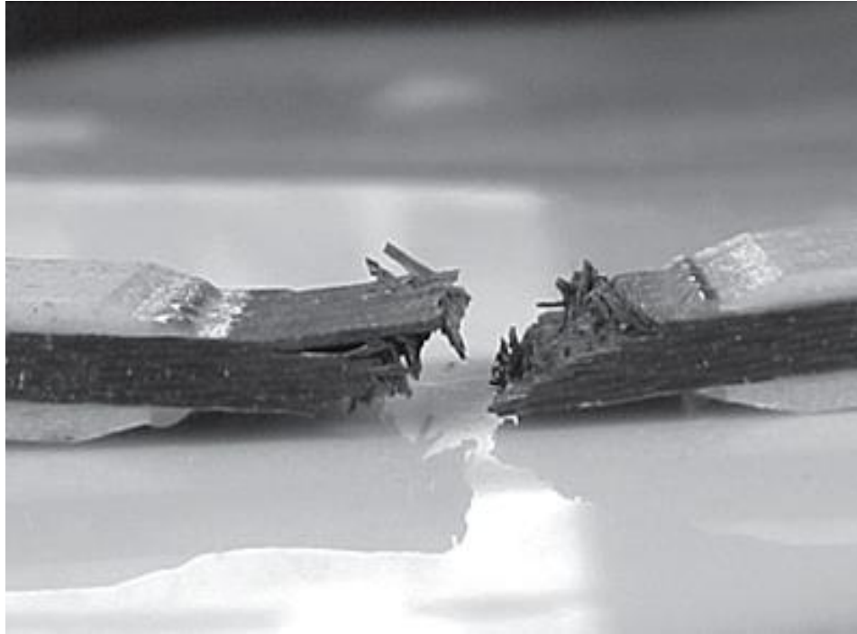
Figure 2.2 F155/PW laminate after compression test showing “shear failure” [22]
