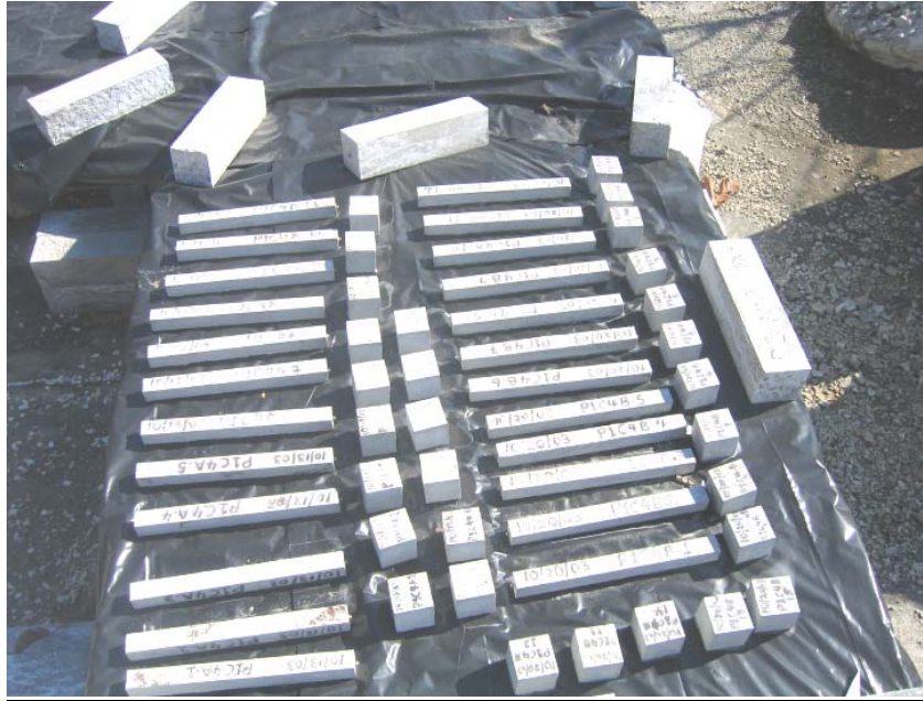
Figure 4.1 Mortar Specimens Exposed to Field Conditions
