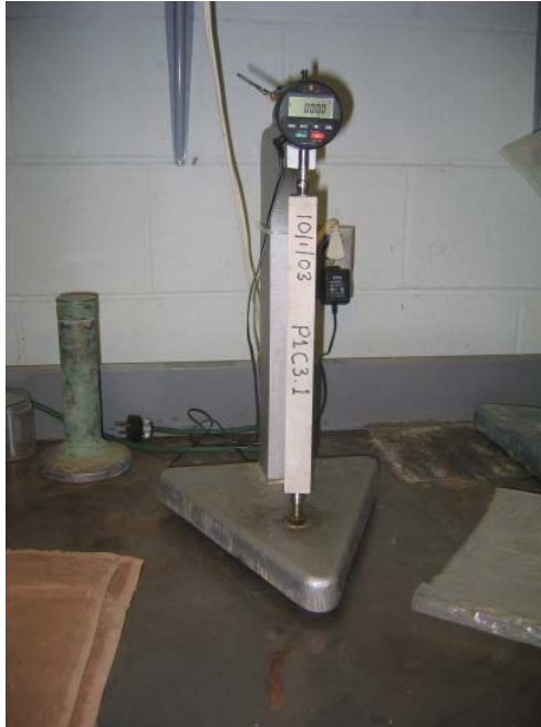
Figure 4.3 Comparator Set up for Length Change Measurements
