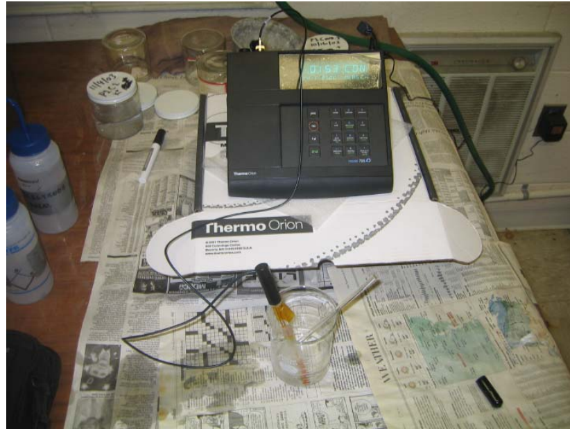
Figure 4.5 ISE and Benchtop Meter Set Up for Water Analysis
