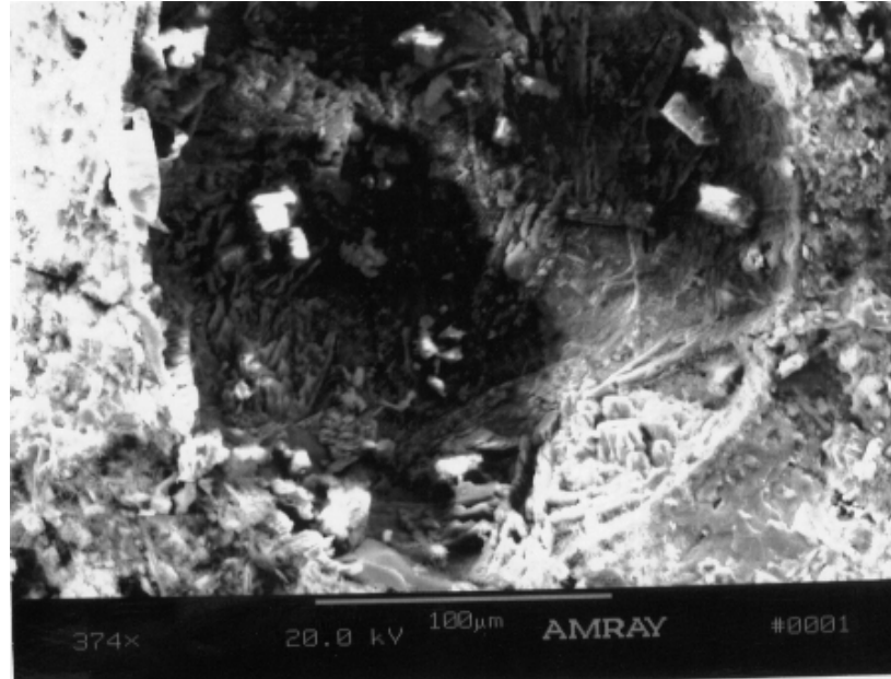
Figure 5.32 SEM Micrograph of Mortar Specimens Under Field Conditions 4B at Age 40 days, Showing Ettringite Needles and CH Crystals within Air Voids
