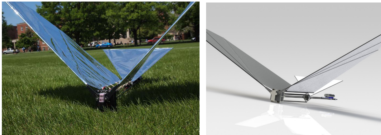
Figure 10 - Fully Assembled Robo Raven (left) and CAD version (right)
