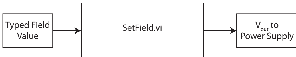
Figure A.3: Set Field ( SetField.vi ) This program sets the field to whatever value is typed into the “Field” text box in the GUI.
