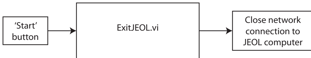
Figure A.10: Close JEOL network connection ExitJEOL.vi This program closes the network connection to the JEOL computer.
