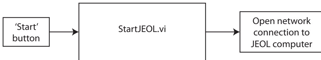
Figure A.9: Open JEOL network connection StartJEOL.vi This program opens the network connection to the JEOL computer. The connection stays open until ExitJEOL.vi is run.
