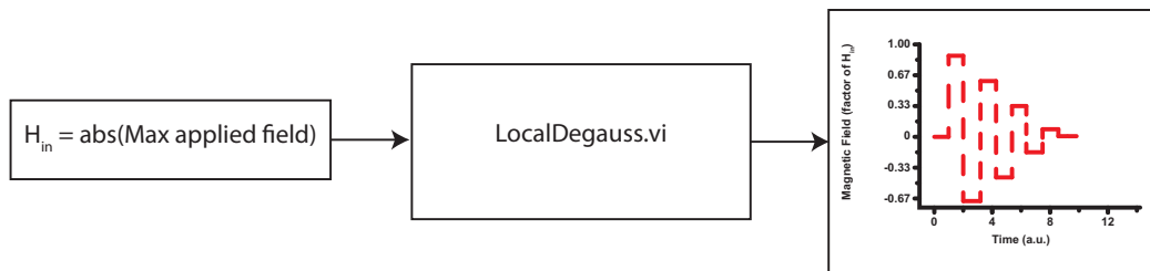
Figure A.2: Local Degauss ( LocalDegauss.vi ) This program is similar to GlobalDegauss.vi except that instead of the starting field being 1 Tesla, it starts from the maximum field magnitude applied. This gives the ability to get the column back to zero field without altering the magnetic state of the sample.
