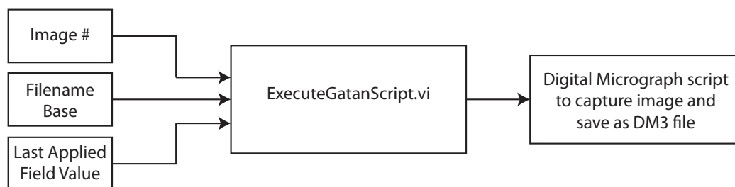
Figure A.6: Execute Digital Micrograph Script ExecuteGatanScript.vi This program concatenates a Digital Micrograph script from the image index, filename base, and last field applied values to capture an image from the CCD and save it to an external hard drive. This script is sent over the network to the computer running Digital Micrograph to run immediately. Note: this program requires the network connection to the Digital Micrograph computer to be open.
