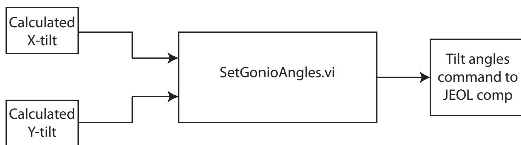
Figure A.5: Set Goniometer Angles (SetGonioAngles.vi) This program reads in the calculated x-tilt and y-tilt values and issues a command over the network to the JEOL TEM control computer to set the x-tilt and y-tilt angles to the calculated values. Note: this program requires the network connection to the JEOL computer to be open.
