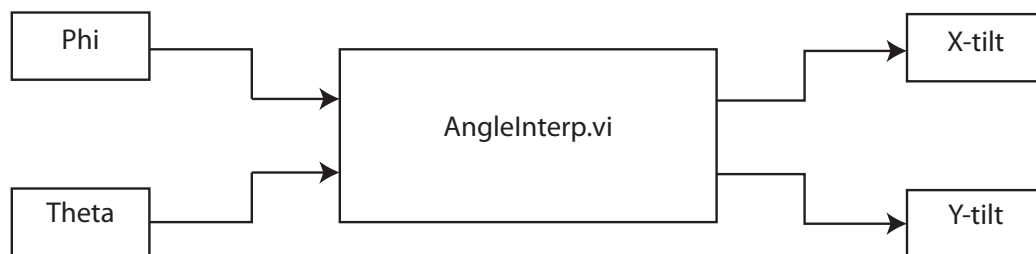
Figure A.4: Angle Interpolation (AngleInterp.vi) This program wraps the \theta and \phi values typed into the GUI such that 0^\circ \leq \phi \leq 360^\circ . It then interpolates the \phi and \theta values typed into the GUI from a few data points that were already calculated and determines the corresponding x-tilt and y-tilt and values.
