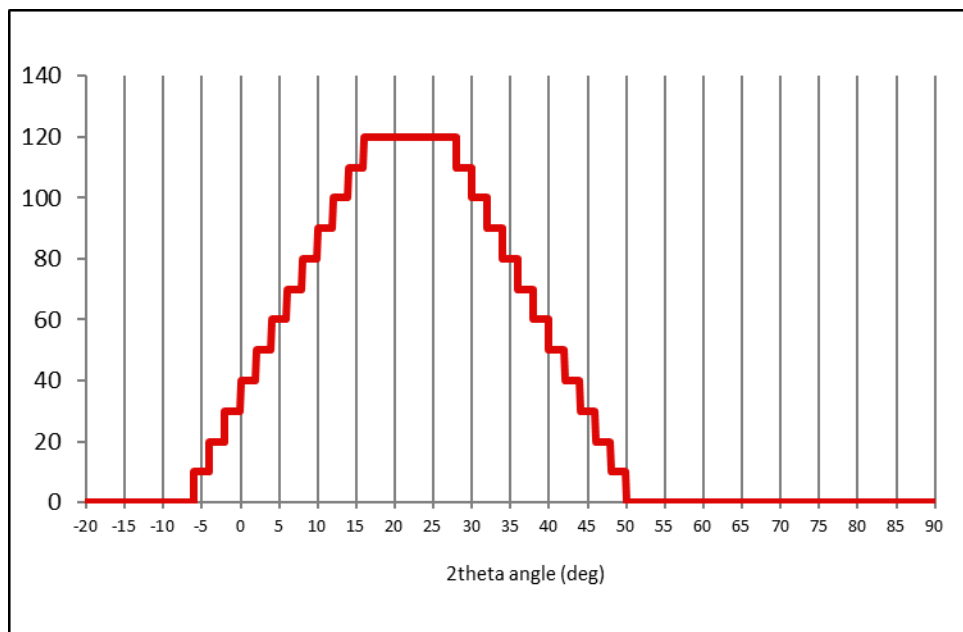
Figure 3.2: Detector coverage time as a function of angle for a standard high resolution scan on 11-BM. The best statistics will be from 22-28°.
