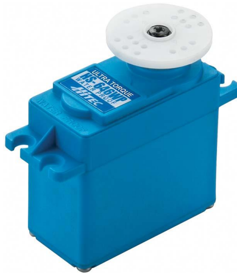
Figure 29: HS-646WP Analog Waterproof High Voltage Servomotor [28]
