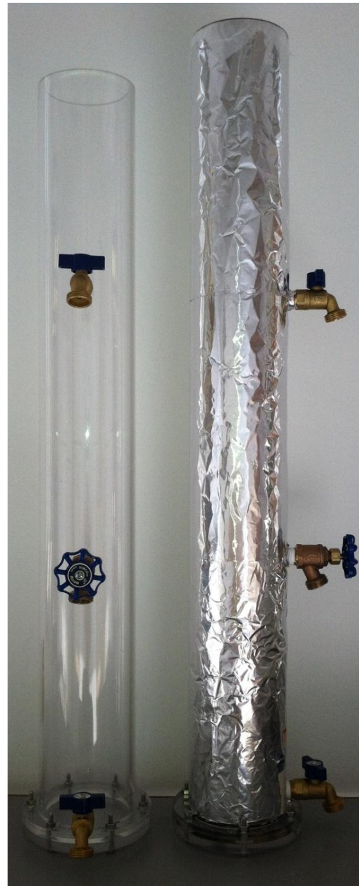
Figure 4: Constructed model bioretention system columns wrapped in aluminum foil to prevent light from entering.
