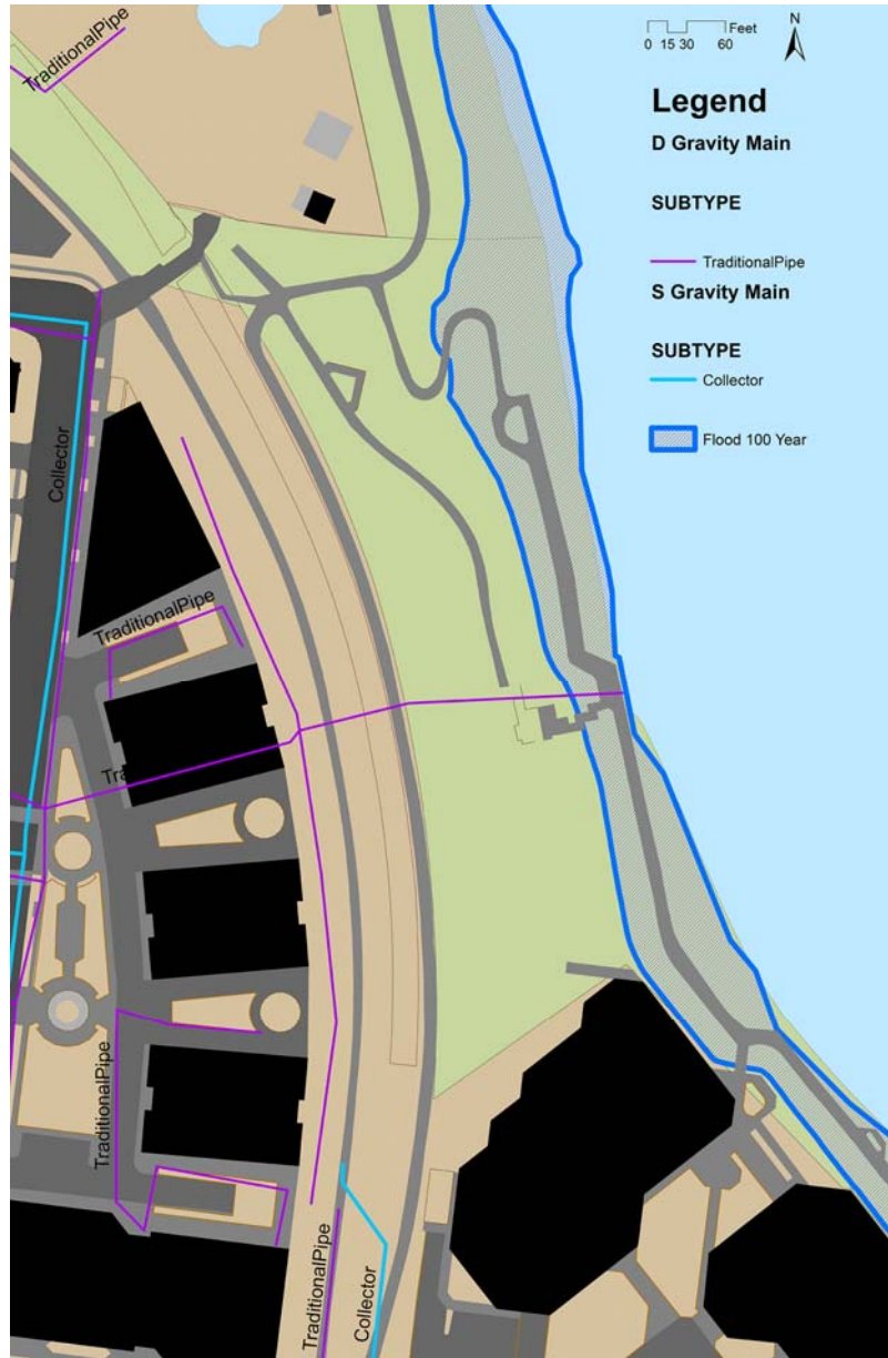
Figure 14: Tide Lock Park storm water pipes and floodplain. Graphic by Erica Thum. GIS data courtesy of the City of Alexandria.
