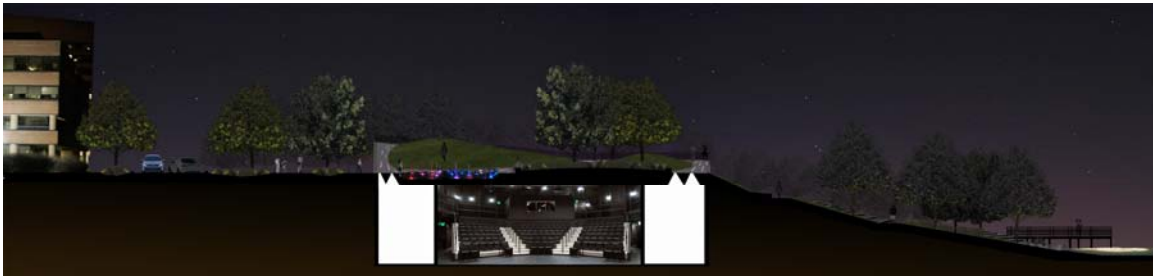
Figure 41: A section cut through the theater building and plaza shows windows in the roof which work as lighting elements both day and night, allowing sun to come in during the day and artificial light to spill out during the night. Drawing by Erica Thum.
