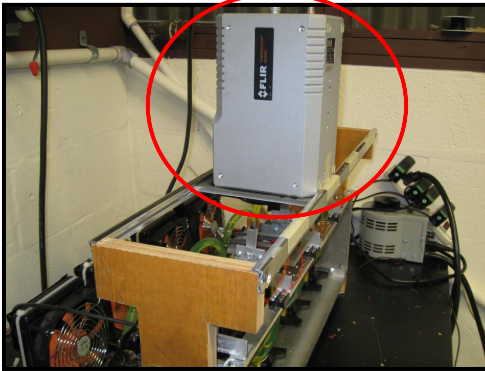
Figure 45: Infrared camera mounted on top of test chassis
