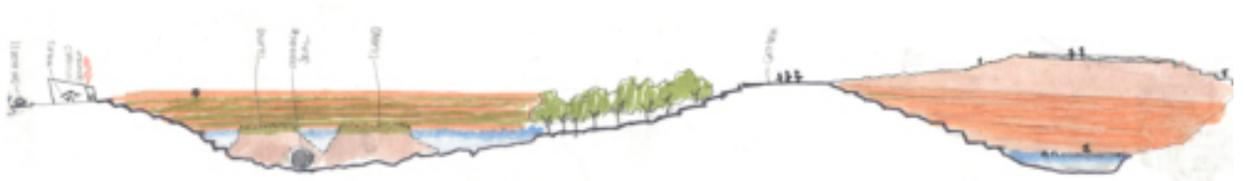
**Figure 20: Section Sketch illustrating the saddle that divides the site, the drainage pipe in the southern gorge and the ephemeral island concept.**
