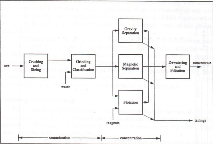
Simplified flow-chart of the beneficiation stage of mining, in which an ore is comminuted and separated into its desired (concentrate) and gangue (tailings) fractions.
